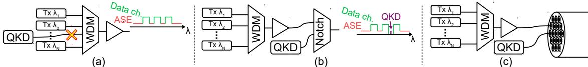
**Fig. 1:** Illustration of multiplexing of QKD and classical channels: (a) EDFAs prohibits QKD channels to use a port of a WDM multiplexer. (b) QKD channels have to be multiplexed after the EDFA where the ASE must be suppressed for the QKD band. (c) System investigated in this paper, QKD channels use a dedicated core to avoid having to employ notch filtering.
