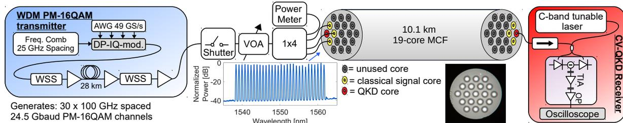
**Fig. 2:** Experimental setup showing: The transmitter generating 30 WDM channels of 24.5 Gbaud PM-16QAM with 100 GHz channel spacing. The multicore fiber with the QKD core surrounded by 3 cores loaded with the classical WDM channels. The QKD receiver based on a balanced photodetector with a C-band tunable laser as local oscillator. The insets show the measured WDM spectra of the classical channels in one core, and the cross section of the MCF used in this experiment.
