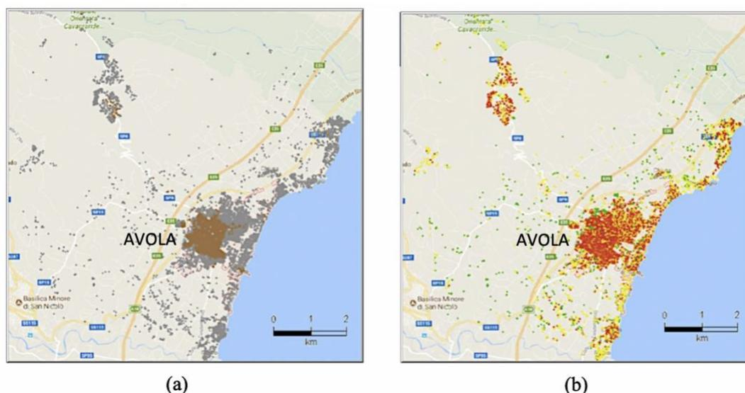
**Figure 4.** Territory of Avola. (a) Geographic Information System (GIS) data set: Masonry (brown) and reinforced concrete (grey) buildings; (b) initial vulnerability map: Low (green), medium (yellow) and high (red) vulnerability buildings.
