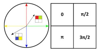
*Fig. S3* The illumination of the pixels is determined by the projection of the desired electric field vector onto the pixel's field vector. The amplitude of the superpixel is the sum of the individual pixel amplitudes and can be any value within a circle in the complex plane. The maximum amplitude possible is equivalent to that generated by ¼ of the pixels illuminated.
