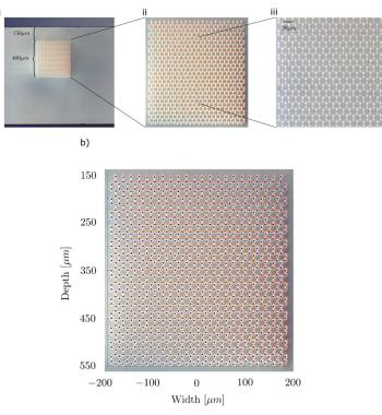
*Fig. S7* a) i)  $10 \times$  microscope image of the end-facet of the silica chip, the lattice is located at  $150 \mu$ m from top surface. The chip is 1.1 mm thick. ii) Zoomed in image, showing the entire lattice. iii)  $40 \times$  microscope image of the centre of the lattice showing the structure of individual wave guides. b) Comparison with desired placement of wave guides. Blue dots mark the designed positions of waveguides.
