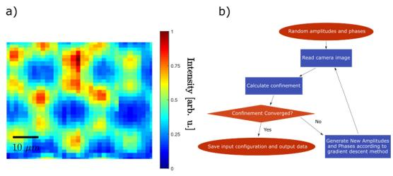
*Fig. S4* a) Total output light intensity plotted as a function of the position of a single x-y scanned input beam. This scan shows the location of waveguides at the input facet. b) Procedure of the optimisation routine maximising the coupling to the vortex zero mode.
