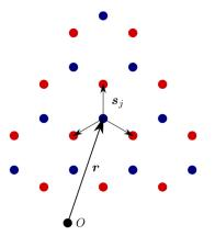
*Fig.* 1 Hexagonal lattice with two triangular sublattices (A and B) in blue and red, lattice vector r and vectors between nearest neighbours  $s_i$  indicated.
