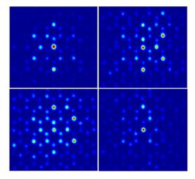
*Fig.* 4 Topological mode with random error distortions. Top left: no error, Top right: maximum 200 nm, Bottom left: maximum 400 nm, Bottom right: maximum 600 nm. The ratios of light intensity in the zero-mode sublattice to the non-mode supporting one are  $\gamma_{AB}$  = 3.8, 2.9, 2.2, 2.1 respectively. The colour map of each image is normalised independently.
