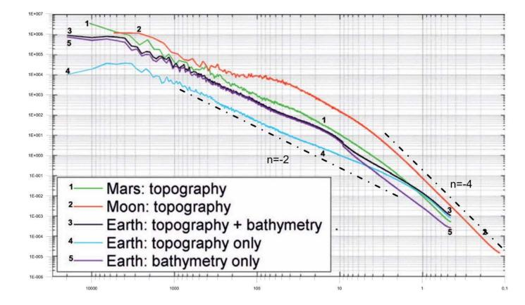
Fig. 2. Relief spectra as functions of the surface wavelength for Moon, Mars and Earth (3 cases labeled at lower left). We added lines  $k^{-2}$  and  $k^{-4}$  for large and small distances.
