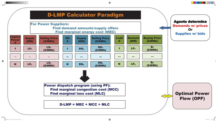
Figure 3.2: General block diagram of DLMP mechanism.
