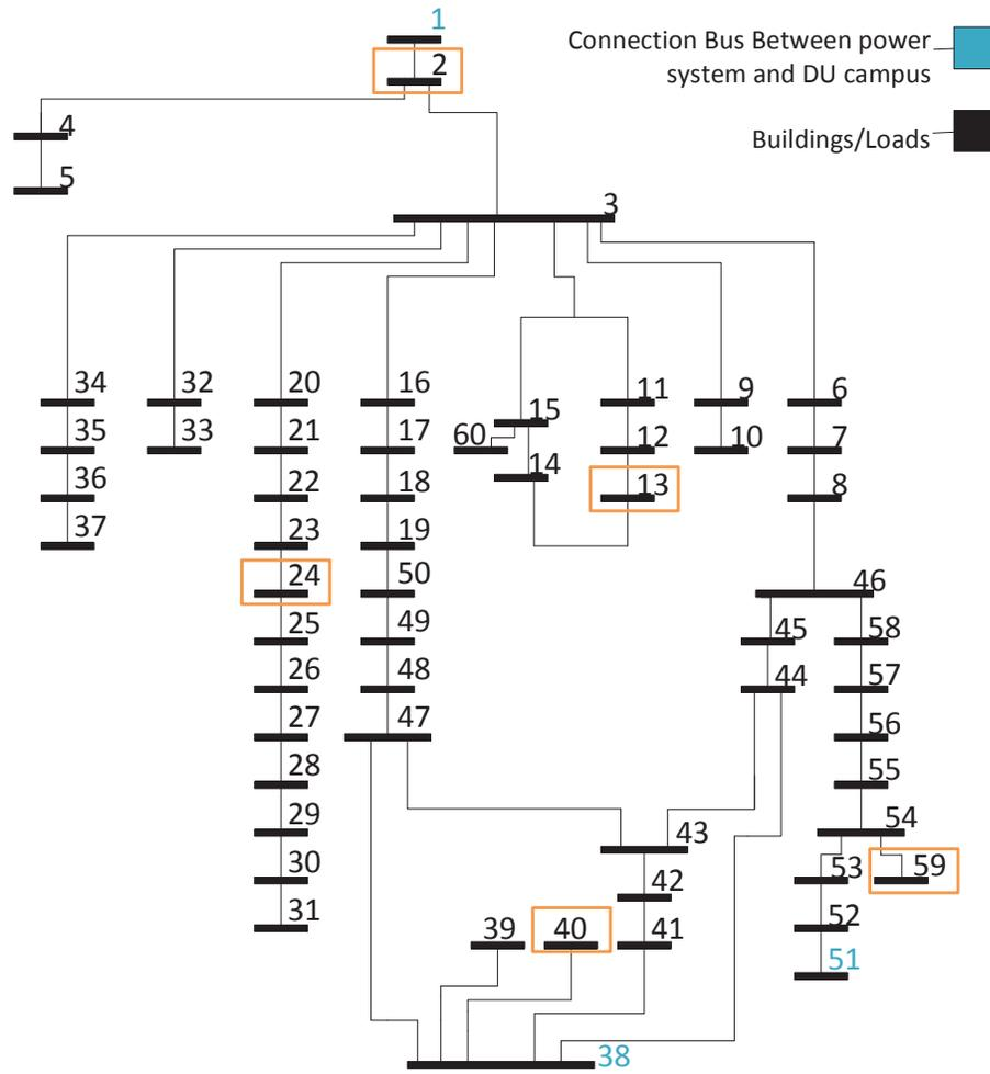
Figure 5.3: The network topology of DU campus grid.
