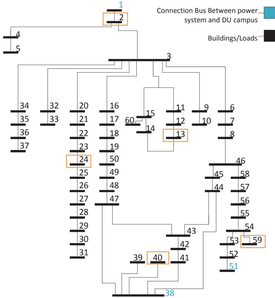
Figure 4.3: The network topology of DU campus grid.
