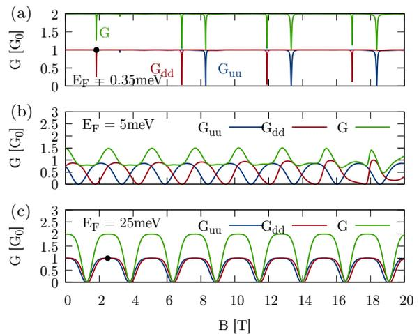
FIG. 6. Conductance of the quantum ring in the (a) QSH regime  $E_F = 0.35$  meV, and in the normal conditions (b,c) for  $E_F = 5$  meV (b) and 25 meV (c) in the absence of vertical electric field.
