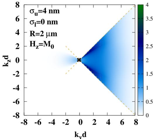
FIG. 6. (Color online) Momentum dependence of the scattering potential  $|\mathcal{B}_{\mathbf{k}K}|$  (in units of  $10^{-8}\mu_0\gamma M_0$ ) between the Kittel mode (marked by a cross) and DE modes with wave vector  $\mathbf{k}$ . The orange dashed curves  $k_z = \pm\sqrt{H_z/M_0}k_y$  is the equal-frequency contour of the DE and Kittel modes that define the boundary between surface and bulk modes [7].
