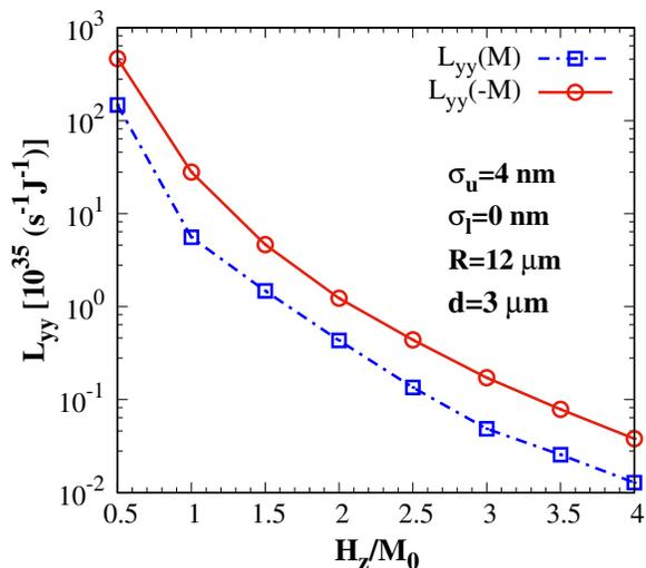
FIG. 5. (Color online) Magnetic-field dependence of spin conductivities  $L_{yy}(\mathbf{M})$  (blue dashed curve with squares) and  $L_{yy}(-\mathbf{M})$  (red solid curve with circles) at the room temperature  $T = 300$  K.
