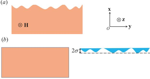
FIG. 1. (Color online) (a) Surface roughness on the upper surface of a magnetic film. The surface normal is along the  $\hat{x}$ -direction. (b) The roughness is located only in a thin surface layer on top of an ordered magnetic film with thickness that corresponds to twice the root-mean-square  $\sigma$  of the thickness fluctuations.
