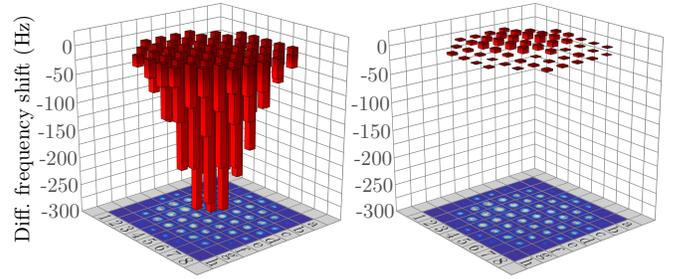
FIG. 1. (Left) Measured differential frequency shift of the ground-state hyperfine splitting of  $^{85}\text{Rb}$  atoms in a two-dimensional array of dipole traps. A fluorescence image of the trapped atom ensembles is shown at the bottom. (Right) Residual frequency shift under identical trapping conditions with a weak additional laser field compensating for the differential light shift.
