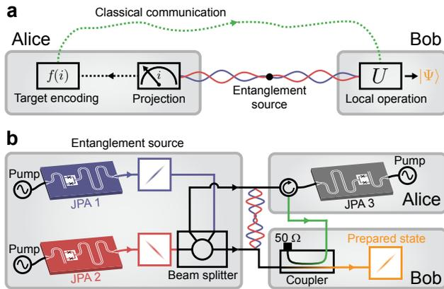
Figure 1. **a** General RSP scheme: Alice remotely prepares a desired state at Bob’s side using a quantum resource and classical communication (feedforward). **b** Experimentally implemented RSP scheme: a two-mode squeezed state (left) serves as quantum resource and the feedforward to Bob (right) is implemented using JPA 3 and a directional coupler.
