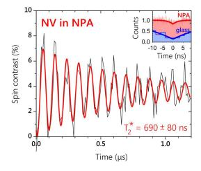
Figure 4. Rabi oscillations detected from a single NV center coupled to a deterministically assembled NPA. The inset shows fluorescence autocorrelation measurements of the NV center in the uncoupled (blue) and coupled (red) configurations.
