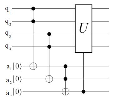
In this diagram, we are performing the general N-control gate strategy. By using three ancilla qubits, we are able to condense the information of all the states stored on our 4-qubit system, down to a single control ancilla. The operator U in the diagram represents any single control gate we've already seen thus far in lesson 3. As an example, let's implement this diagram in code, replacing U with a control-Z gate:
