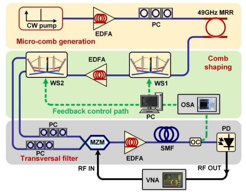
Fig. 1. Schematic diagram of the 80-tap photonic RF transversal filter based on an integrated 49GHz-spacing micro-comb source. EDFA: erbium-doped fiber amplifier. PC: polarization controller. MRR: micro-ring resonator. WS: Waveshaper. MZM: Mach-Zehnder modulator. SMF: single mode fiber. OC: optical coupler. OSA: optical spectrum analyzer. PC: computer. PD: photodetector. VNA: vector network analyzer.
