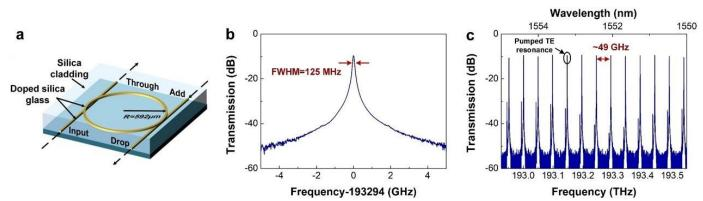
Fig. 2. (a) Schematic illustration of the integrated MRR for generating the Kerr micro-comb. (b) A resonance at 193.294 THz with full width at half maximum (FWHM) of 124.94 MHz, corresponding to a quality factor of  $1.549 \times 10^6$ . (c) Drop-port transmission spectrum of the integrated MRR with a span of 5 nm, showing an optical free spectral range of 49 GHz.
