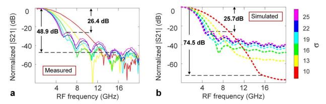
Fig. 7. (a) Measured and (b) simulated RF transmission spectra of the Gaussian-apodized sinc filter.
