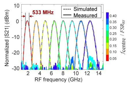
Fig. 9. Measured and simulated RF transmission spectra of the centre-frequency-tunable Gaussian apodized sinc filter
