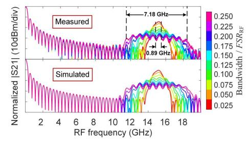
Fig. 12. Measured and simulated RF transmission spectra of the all-positive-tap bandwidth-tunable filter.
