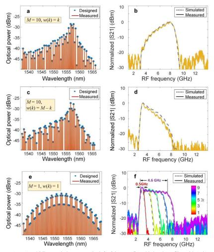
Fig. 10. Shaped micro-comb spectra (a, c, e) and RF transmission spectra (b, d, f) of the reconfigurable bandpass filter with (a, b) a positive transmission slope, (c, d) a negative transmission slope, and (e, f) varying bandwidth.
