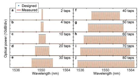
Fig. 4. Optical spectra of the shaped micro-comb corresponding to the tap weights of a sinc filter with different tap number.
