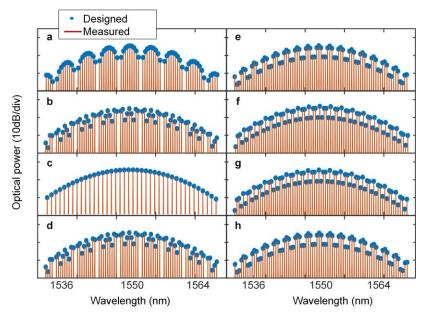
Fig. 8. Optical spectra of the shaped micro-comb corresponding to the centre-frequency-tunable Gaussian apodized sinc filter. (a-h) corresponds to a designed centre frequency ranging from  $0.05 \times FSR_{RF}$  to  $0.40 \times FSR_{RF}$ , with a step of  $0.05 \times FSR_{RF}$ .
