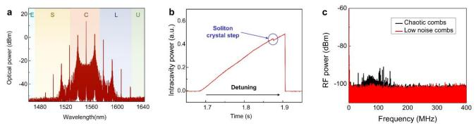
Fig. 3. (a) Optical spectrum of the generated micro-combs with 200 nm span. (b) Measured transmission of a single resonance showing the soliton crystal step, and (c) the measured RF spectra.
