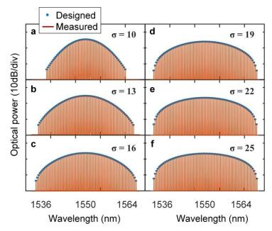
Fig. 6. Optical spectra of the shaped micro-comb corresponding to the Gaussian-apodized sinc filter. (a-f) corresponds to the root mean square width of the Gaussian function  $\sigma$  set from 10 to 25, with a step of 3.
