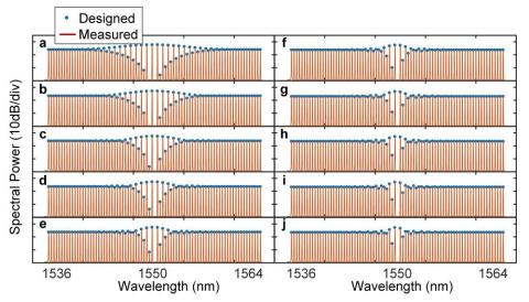
Fig.11. Optical spectra of the shaped micro-comb corresponding to the all-positive-tap bandwidth-tunable filter. (a-j) corresponds to a designed bandwidth from  $0.025 \times FSR_{RF}$  to  $0.25 \times FSR_{RF}$ , with a step of  $0.025 \times FSR_{RF}$ .
