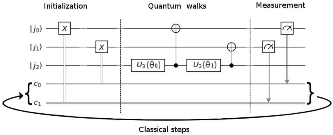
FIG. 2: Discrete-time coined quantum walk circuit for the  $4 \times 4$  transition matrix given in Eq. (10). Qubits  $j_0$  and  $j_1$  are state register qubits to represent the four-node graph in Fig. 1, first set as 0 before initialization, while the qubit  $j_2$  is the coin register qubit. The measured registers  $c_0$  and  $c_1$  are fed back to initialize the next iteration. The classical-step is repeated  $c$  times to obtain the Neumann expansion up to order  $c$ .
