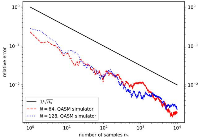
FIG. 4: Relative errors  $\epsilon = |x_I^{exact} - x_I|/|x_I^{exact}|$  as a function of the sampling number  $n_s$  for  $N = 64$  and  $N = 128$  matrices, obtained by performing two quantum walk evolutions,  $\mathcal{U}^2$ . Black solid lines represent the  $1/\sqrt{n_s}$  error reduction expected for Monte Carlo calculations. Red dashed line and blue dotted line are the results computed by the QASM simulator.
