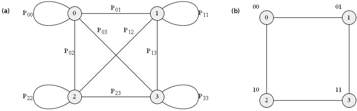
FIG. 1: (a) Quantum (or classical) random walk on an undirected  $N = 4$  graph. The transition probability of going from node  $I$  to node  $J$  or vice versa is equal to  $P_{I,J}$ , these elements forming a  $4 \times 4$  matrix. (b) The four nodes on this Hamming cube are labeled by integers (0, 1, 2, 3); they are encoded as four different states  $|00\rangle$ ,  $|01\rangle$ ,  $|10\rangle$ ,  $|11\rangle$ , respectively.
