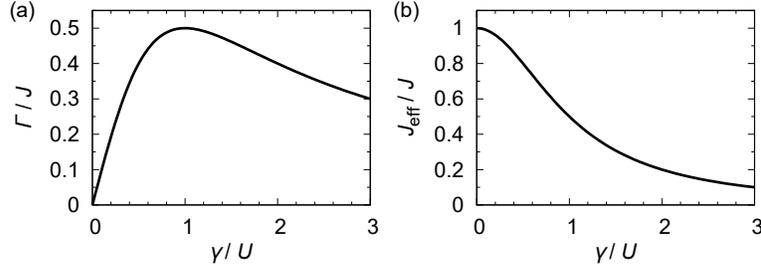
FIG. S1. (a)  $\gamma$ -dependence of the imaginary part of the effective spin-exchange interaction. (b)  $\gamma$ -dependence of the real part of the effective spin-exchange interaction. Here  $J$  is given by  $J = 4t^2/U$ .
