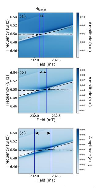
Fig. 6. Spectra plus identified peaks (black, dotted line) for  $\delta_0 = 1.31$  [(a)],  $\delta_0 = 2.15$  [(b)], and  $\delta_0 = 2.71$  [(c)]. We found from simulations, confirming a finding from Ref. [23], that this distance corresponds to  $4\Im g'(\delta_0,\phi)$ . As the cavity port is more and more attenuated, the relative strength of the contribution from direct crosstalk increases which is seen by the anticrossing like behavior around resonance.
