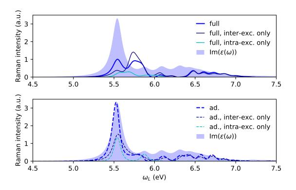
Figure 3: **hBN: Raman intensity with only inter- or intra-exciton scattering.** Raman intensity with all contributions (thick lines) and with only inter- or intra-exciton scattering (darker and lighter thin lines, respectively) taken into account. Top panel: full, non-adiabatic case. Bottom panel: adiabatic limit. The shaded area represents the absorption spectrum. The Raman intensity is given in the same units in both panels and as in Fig. 1.
