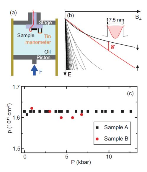
Fig. 1 Introduction. (a) Experimental setup of the hydrostatic pressure cell. (b) Typical Landau level diagram of 2D holes confined in symmetric, narrow quantum wells. Due to the strong SOI, the Landau levels are non-linear with *B*. The character of the lowest two Landau levels (the thick black and red curves), which are relevant to our observations, are predominately the N = 0 harmonic oscillators with  $\uparrow$  and  $\downarrow$  pseudospins. (c) The measured
