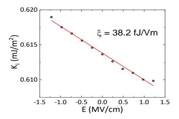
Figure S4. Interfacial anisotropy ( $K_i$ ) as a function of the applied electric field (E) in the sample with CoFeB thickness of 1.06 nm. The slope of this plot is the VCMA coefficient ( $\xi$ ).
