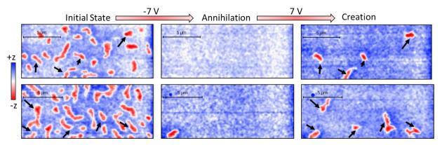
Figure 2. MFM images obtained before and after application of electric field. Left column: magnetization state before application of any electric field. Middle Column: Magnetization state obtained after applying a negative voltage pulse that increased PMA. Right Column: Magnetization state obtained after applying a positive voltage pulse that decreased PMA.
