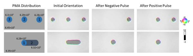
Figure 4. Top panel: Skyrmion annihilation and creation by VCMA. The numbers show the PMA in J/m<sup>3</sup>. Pinning strength: 1>2>3. Bottom Panel: Creation of skyrmion from a chiral domain.
