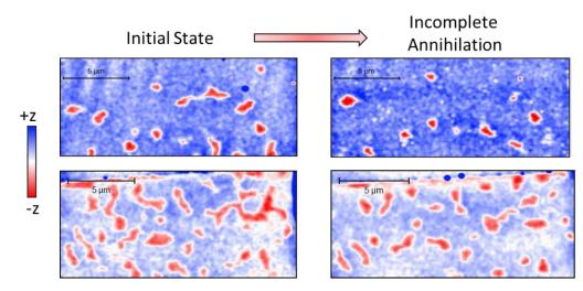
Figure S7. Other examples of incomplete annihilation due to a negative voltage pulse
