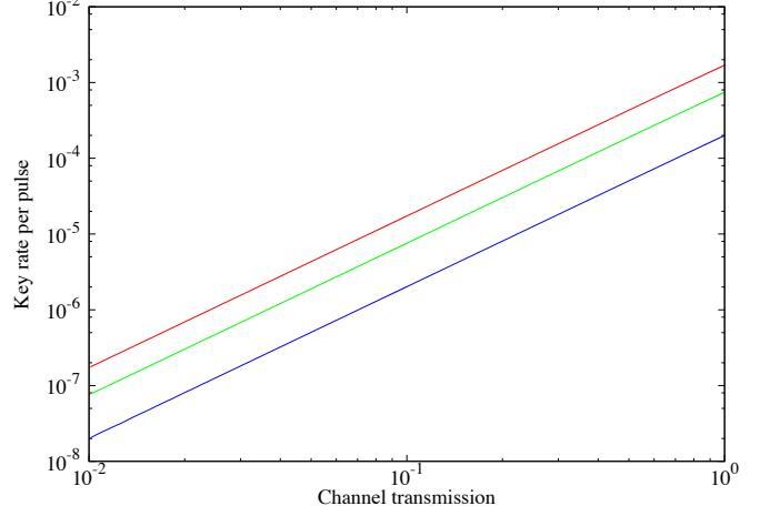
FIG. 2: Secure key rate  $R$  per pulse as a function of the overall channel transmission  $\eta$ . The top, the middle and the bottom lines respectively represent the key rates for  $e_{\text{bit}} = 0.01$ ,  $e_{\text{bit}} = 0.02$  and  $e_{\text{bit}} = 0.03$ .
