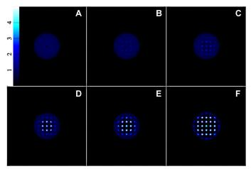
Fig. 6. Snapshots of the density on a linear scale during the onset of crystallization. Panels (**A**) to (**C**) correspond to points 19, 20, and 21, respectively, on Fig. 5. The later stages of crystallization are shown in panels (**D**) to (**F**) corresponding to points 25, 30, and 49, respectively, on Fig. 5.
