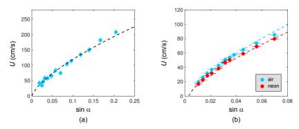
**Figure 3.** Water drop mobility on SH inclines. In all plots, the drop volume is  $\Omega = 100 \,\mu\text{L}$  and dashed lines show Eq. 3. (a) Terminal velocity U as a function of the sine of the sliding angle  $\alpha$  for water drops. (b) Terminal velocity U as a function of sin  $\alpha$  for water drops in an atmosphere of air (light blue circles) or neon (red circles).
