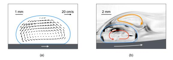
**Figure S3. (a)** PIV visualisation of the flow inside a 100  $\mu$ L water drop placed in a rotating cylinder moving at 0.26 m/s. The fluid is observed to be in rotation as assumed in our model. **(b)** Smoke visualization of the gas flow around the drop (the image displayed is the standard deviation obtained from the high-speed imaging of the phenomenon). A vortex (orange arrow) rotating in the opposite rolling direction (red arrow) is observed to stay attached to the drop.
