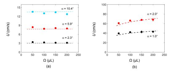
**Figure S2.** Terminal velocity *U* of drops as a function of their volume  $\Omega$  for various tilting angles  $\alpha$ . We present data in the viscous regime (a,  $\eta = 110$  mPa.s) and in the inviscid regime (b,  $\eta = 1$  mPa.s). Dashed lines represent Eq. 3 with x = 0.85 and y = 34.
