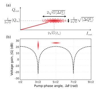
FIG. 26. Phase-sensitive parametric amplification. (a) In contrast to the phase-insensitive operation, phase-sensitive parametric amplification allows us to suppress the noise along one axis. Consequently, the noise is added to the other quadrature. (b) Voltage gain as a function of pump-phase angle, in which the amplification depends on the phase of the pump, providing either amplification or de-amplification of the quadrature voltage.
