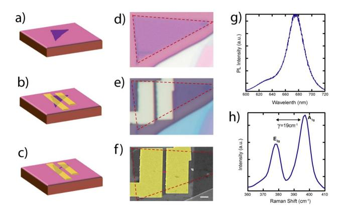
Figure 1. Schematic of fabrication process for NR based field effect transistor in single layer  $MoS_2$  (a-c). Schematic of the device fabrication showing step-by-step process going from a  $MoS_2$  flake (triangle) to nanoribbon (NR) device where yellow stripes are the metallic contacts. (d-f) actual device images showing step-by-step process corresponding (a-c). Scale bar in panel (f) is 1 $\mu$ m. (g, h) shows PL and Raman spectroscopy respectively to validate single layer  $MoS_2$ .
