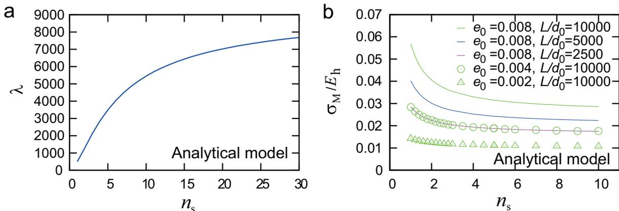
FIG. 3: (a) The common enhancement factor for the fracture toughness and strength as a function of  $n_s$ , obtained from the scaling law in Eq. (7). (b) The maximum stress that appears at a crack tip as a function of  $n_s$ , obtained from the result of our scaling analysis given in Eq.(8) setting the numerical factor for the relation to be 1.
