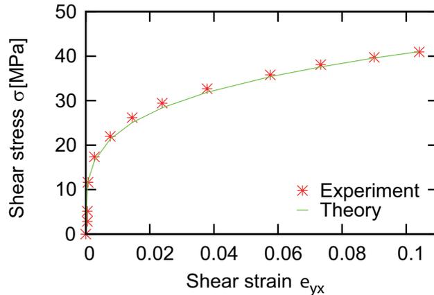
FIG. 2: Comparison of an experimentally obtained stress-strain curve (red star symbols) for shear deformation in [24] with a stress-strain curve obtained with our analytical model (solid line) shows close agreement.
