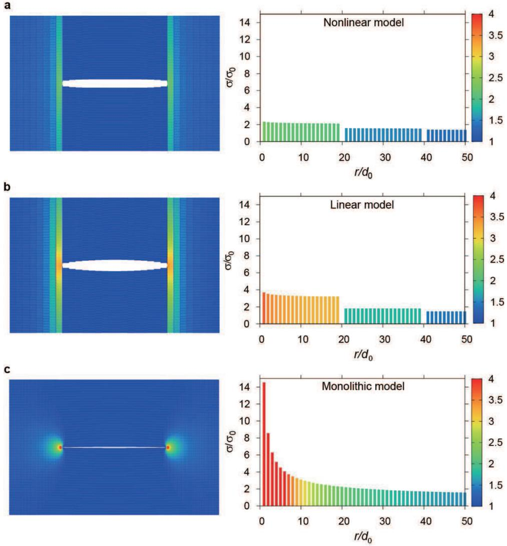
FIG. 4: Comparison of stress distribution with the three models: (a) Nonlinear model mimicking nacre. (b) Linear model. (c) Monolithic model. (left) Stress distribution around a crack in the network model composed of  $960 \times 10000$  grid points. (right) Stress along the  $x$  axis as a function of distance from the crack tip.
