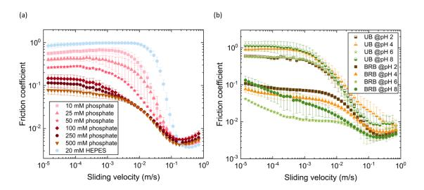
Fig. 2 Stribeck curves as a function of the sliding velocity. The data shown was obtained with different buffer solutions on a steel-PDMS material pairing: (a) 10 mM phosphate, 25 mM phosphate, 50 mM phosphate, 100 mM phosphate, 250 mM phosphate, 500 mM phosphate and 20 mM HEPES. (b) UB and BRB at different pH levels (from pH 2 to 8). Error bars denote the standard deviation as obtained from n = 3 different measurements.
