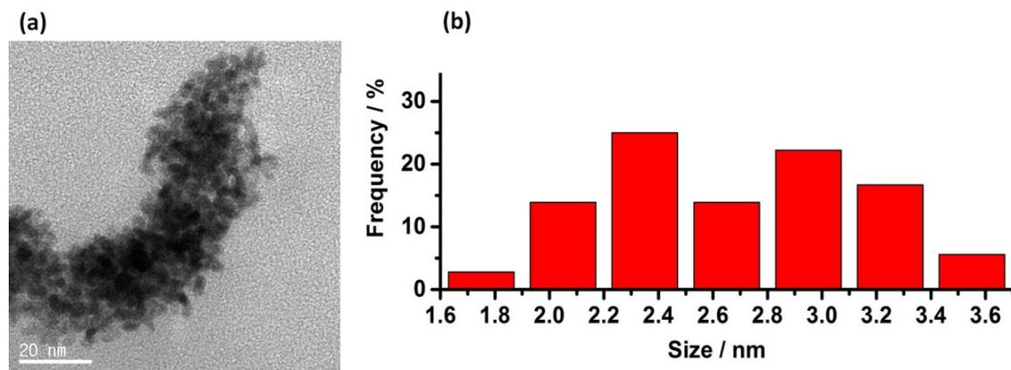
**Figure S27.** (a) TEM image of Pt/CTAB and (b) the corresponding size distribution histogram of Pt nanoparticles ( $2.7 \pm 0.3$  nm).
