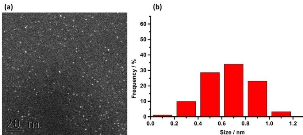
**Figure S12.** (a) HAADF-STEM image of Au clusters in an acid solution (pH=3) and (b) the corresponding size distribution histogram of Au clusters.
