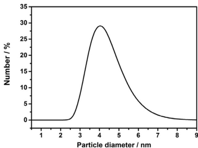
**Figure S21.** The number-average size distribution of the Au@I-Cage-TFSI in EA solution observed by DLS.
