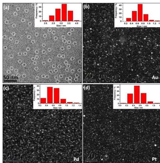
**Figure 1.** (a) Cryo-EM image of Au@I-Cage-Cl on a Lacey carbon grid and the size distribution histogram. Some Au@I-Cage-Cl are highlighted by white dotted circles. (b-d) HAADF-STEM images and the size distribution histograms of Au, Pd and Pt clusters, respectively.
