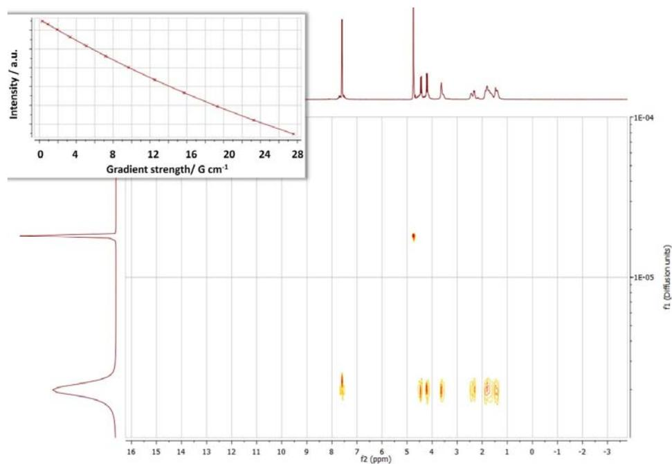
**Figure S10.**  $^1\text{H}$  2D-DOSY NMR spectrum of Au@I-Cage-Cl in  $\text{D}_2\text{O}$ . The inset in upper left is the plot of the signal intensity as a function of the gradient strength. Diffusion coefficients are obtained by non-linear fitting of the decay curve.
