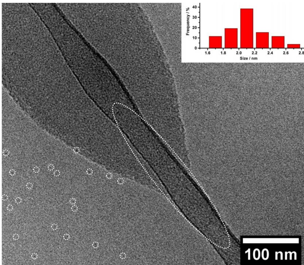
**Figure S5.** Cryo-EM image of the neutral RCC3 Cage (some dots highlighted by white circles) on a Lacey carbon grid. There are also a large number of RCC3 cage on Lacey carbon (highlighted by white dotted ellipses). The inset is the corresponding size distribution histogram of RCC3 cage.
