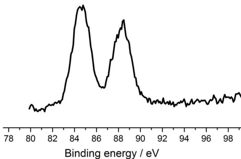
**Figure S8.** XPS spectrum of Au@I-Cage-Cl showing Au  $4f_{7/2}$  (84.4 eV) and  $4f_{5/2}$  (88.4 eV) peaks of metallic Au.
