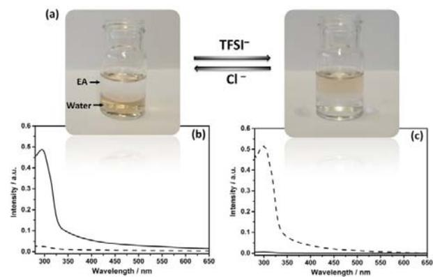
**Figure 2.** (a) Photographs showing reversible transfer of Au-I-Cage-X ( $X = \text{Cl}^-$  or  $\text{TFSI}^-$ ) between aqueous and EA phases upon anion exchange. (b, c) UV-Vis spectra of Au clusters transferred between aqueous and EA phases (solid curve for aqueous phase, dotted curve for EA phase) as shown in (a).
