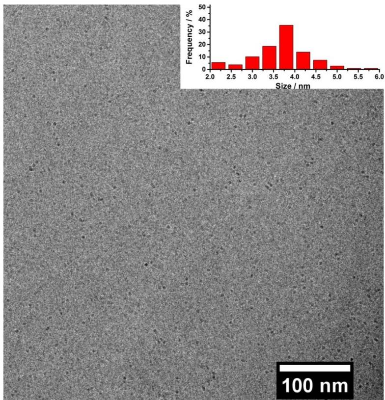
**Figure S22.** Cryo-EM image of Au@I-Cage-TFSI on a Lacey carbon grid and the size distribution histogram as inset.
