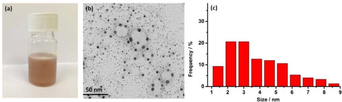
**Figure S17.** (a) Photograph of Au/RCC3 solution. (b) TEM image of Au/RCC3 and (c) the corresponding size distribution histogram of Au nanoparticles ( $4 \pm 0.8$  nm).
