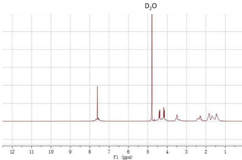
**Figure S40.** The <sup>1</sup>H NMR spectrum of the Pt@ I-Cage-Cl in D<sub>2</sub>O.
