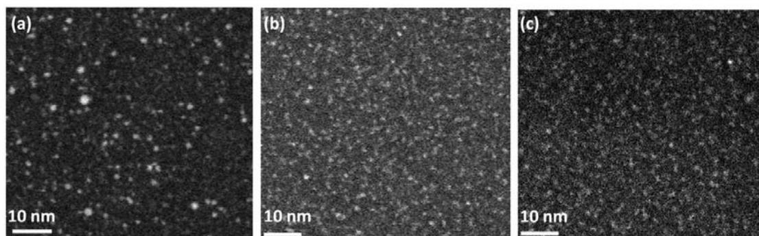
**Figure S7.** The HAADF-STEM images of (a) Au, (b) Pd and (c) Pt clusters in aqueous solution.
