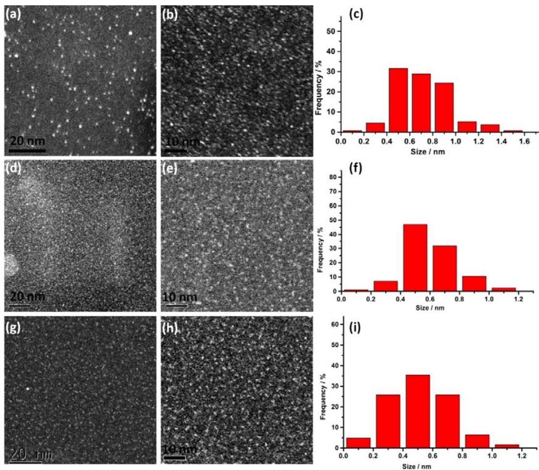
**Figure S23.** HAADF-STEM images at different magnifications and their corresponding size distribution of Au (a-c), Pd (d-f) and Pt (g-i) clusters in EA solution.
