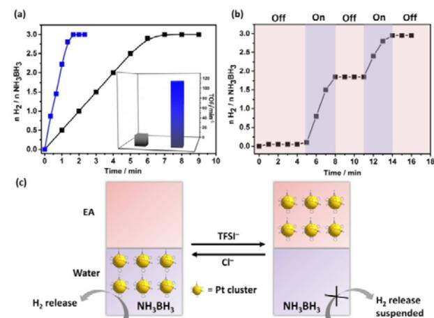
**Figure 3.** (a) Time course plots of  $\text{H}_2$  generation for the hydrolysis of ammonia borane (AB) over the Pt@I-Cage-Cl (blue line) and unsupported Pt catalysts, Pt-SP-Free (dark line) at 300 K ( $\text{Pt}/\text{AB} = 0.02$ ). Inset: the corresponding TOF values. (b) Control of  $\text{H}_2$  release in the AB hydrolysis in water-EA mixture (pink and violet regions for "off" and "on" state, respectively). (c) Diagram of controlled  $\text{H}_2$  release process.
