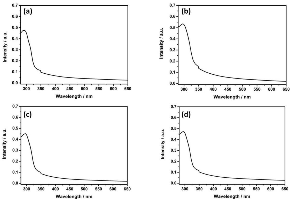
**Figure S11.** UV-vis spectra of Au cluster after staying in (a) acid, (b) base, (c) heat-treatment at 363 K and (d) liquid N<sub>2</sub>.
