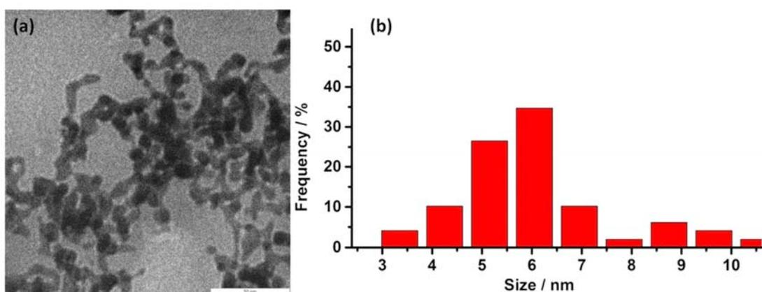
**Figure S18.** (a) TEM image of Au/4-cyanomethyl-1-vinyl-imidazolium bromide and (b) the corresponding size distribution histogram of Au nanoparticles ( $6 \pm 0.9$  nm).
