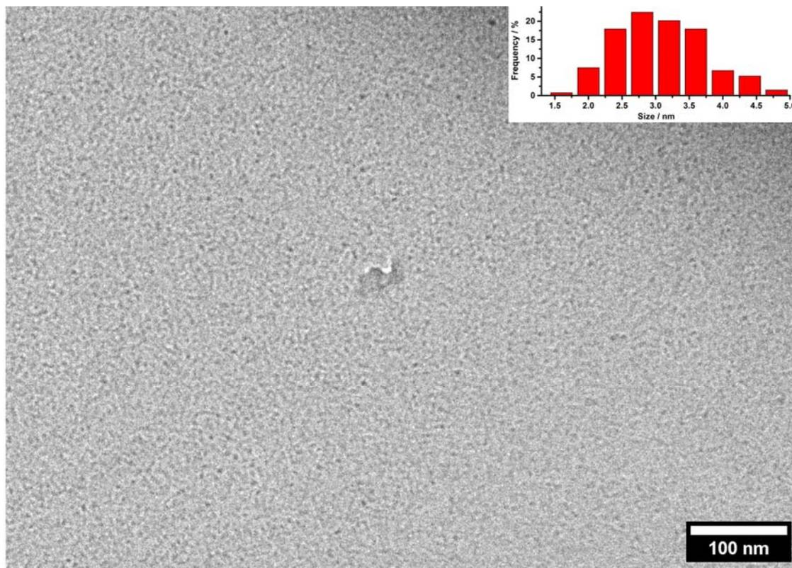
**Figure S4.** Cryo-EM image of the I-Cage-C1 (dark dot) on a Lacey carbon grid. The inset is the corresponding size distribution histogram of I-Cage-C1.
