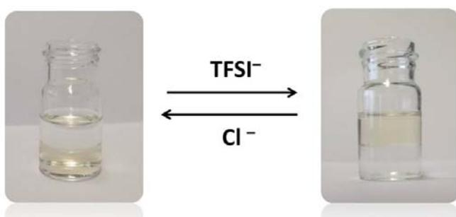
**Figure S24.** Photographs of the reversible phase transfer of Pd clusters assisted by the cage molecules between an aqueous and EA phases upon anion exchange.
