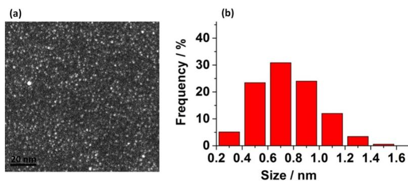
**Figure S26.** (a) HAADF-STEM image of Pt@I-Cage-Cl catalyst and (b) the corresponding size distribution histogram of Pt clusters ( $0.75 \pm 0.2$  nm).
