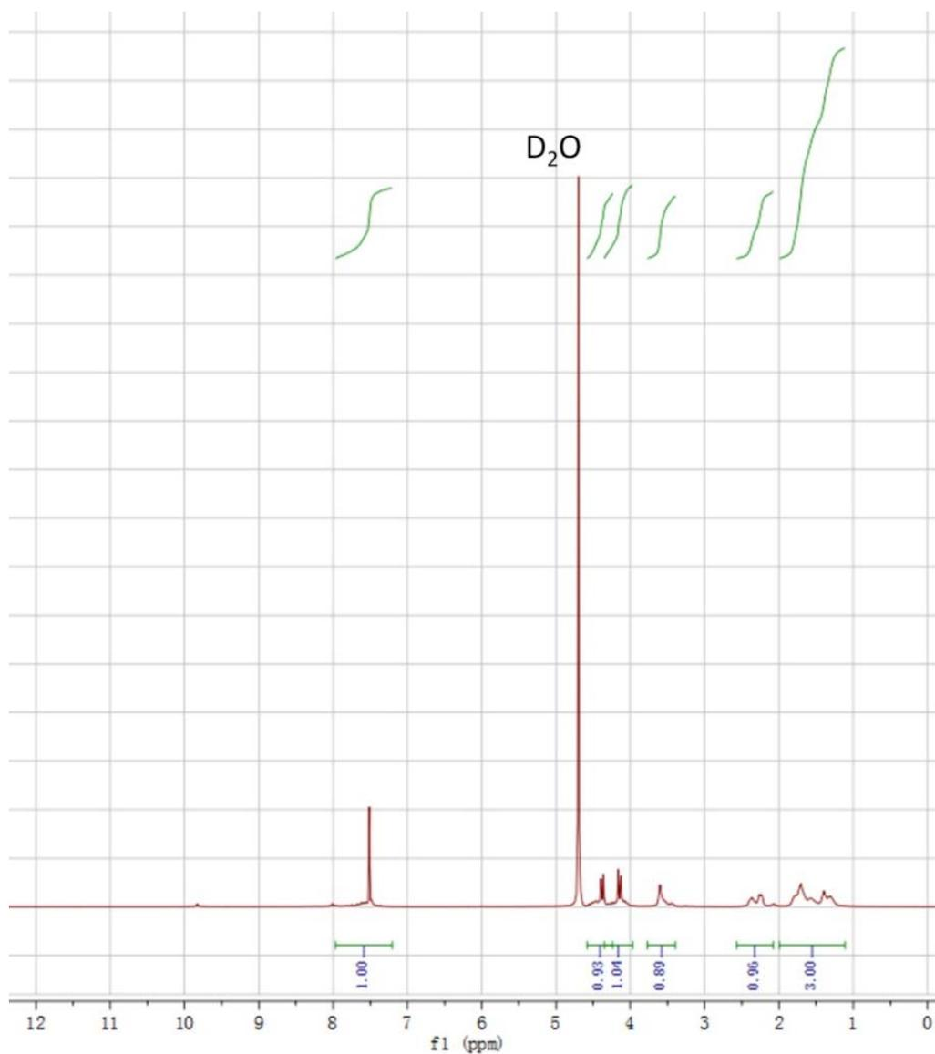
**Figure S38.** The integration of the  $^1\text{H}$  NMR spectrum of the I-Cage-Cl in  $\text{D}_2\text{O}$ .
