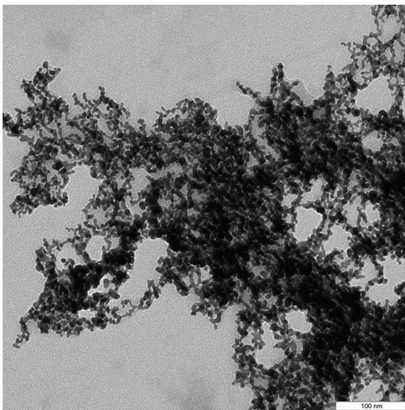
**Figure S16.** TEM image of Au nanoparticles produced without any support.
