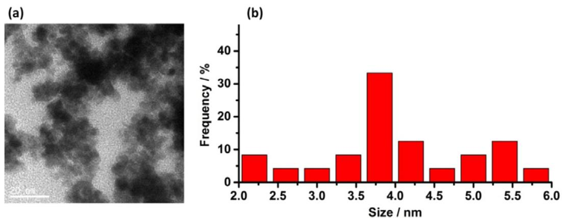
**Figure S29.** (a) TEM image of Pt/PVP and (b) the corresponding size distribution histogram of Pt nanoparticles ( $4 \pm 0.4$  nm).
