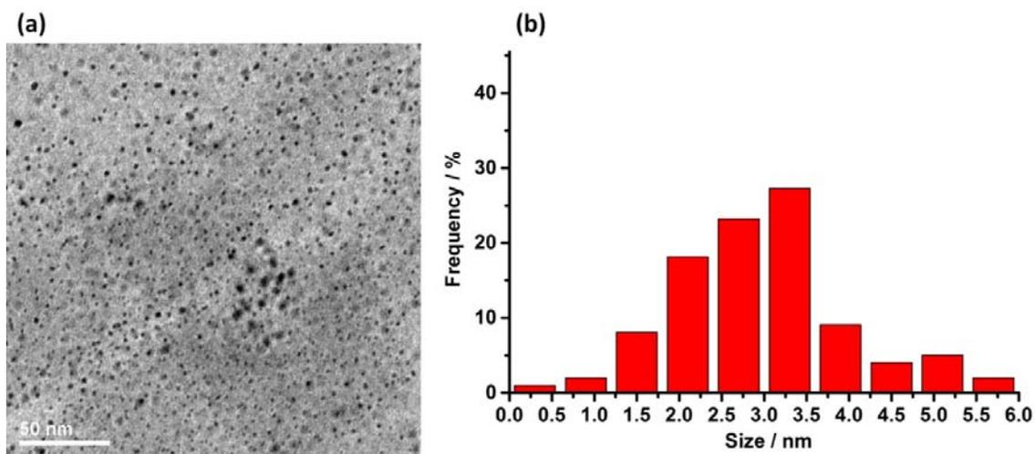
**Figure S31.** (a) TEM image of Pt/RCC3 and (b) the corresponding size distribution histogram of Pt nanoparticles ( $3 \pm 0.6$  nm).
