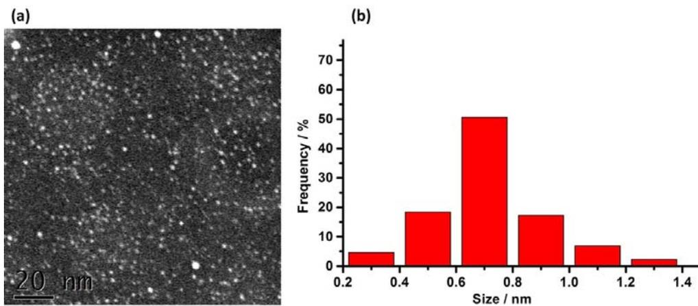
**Figure S15.** (a) HAADF-STEM images of Au cluster after heat-treatment at 363 K and (b) the corresponding size distribution histogram of Au clusters.
