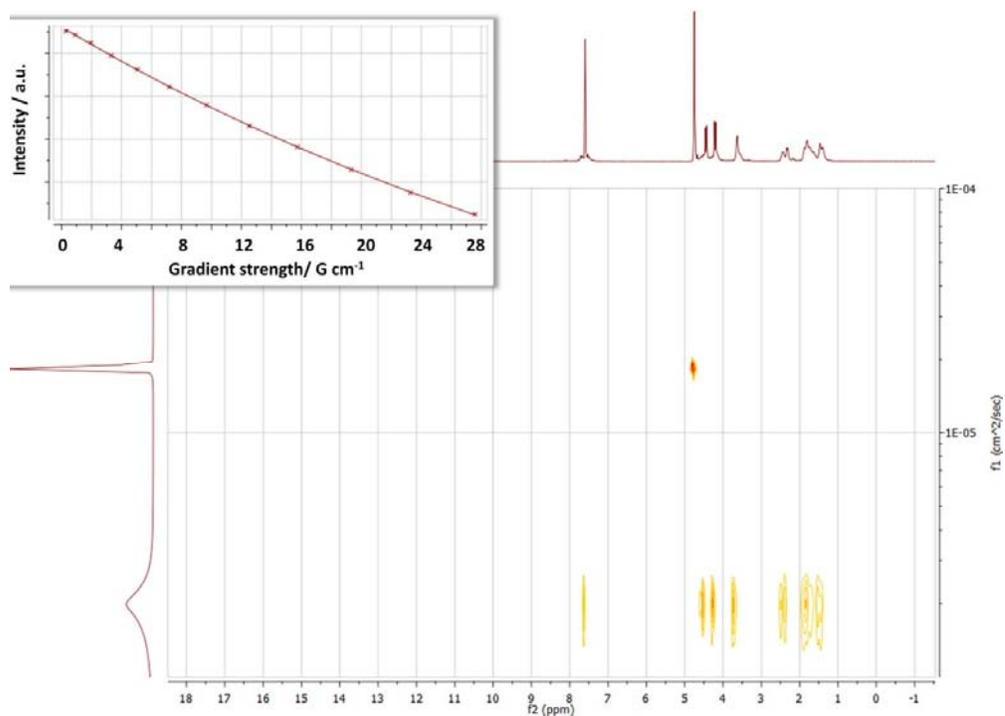
**Figure S9.**  $^1\text{H}$  2D-DOSY NMR spectrum of I-Cage-Cl in  $\text{D}_2\text{O}$ . The inset in upper left is the plot of the signal intensity as a function of the gradient strength. Diffusion coefficients are obtained by non-linear fitting of the decay curve.
