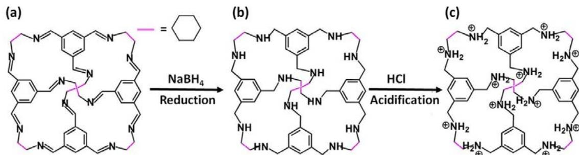
**Scheme S1.** Scheme illustrating the procedure to prepare the ionic organic cage (I-Cage) from its CC3 precursor, (a) CC3, (b) R-CC3, and (c) I-Cage-Cl (The  $\text{Cl}^-$  counter anions are omitted for clarity).
