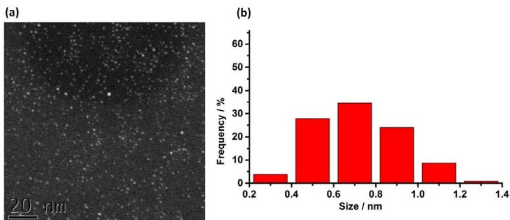
**Figure S14.** (a) HAADF-STEM image of Au clusters after treated by liquid nitrogen and (b) the corresponding size distribution histogram of Au clusters.
