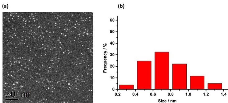
**Figure S13.** (a) HAADF-STEM image of Au clusters in a base solution (pH=10) and (b) the corresponding size distribution histogram of Au clusters.
