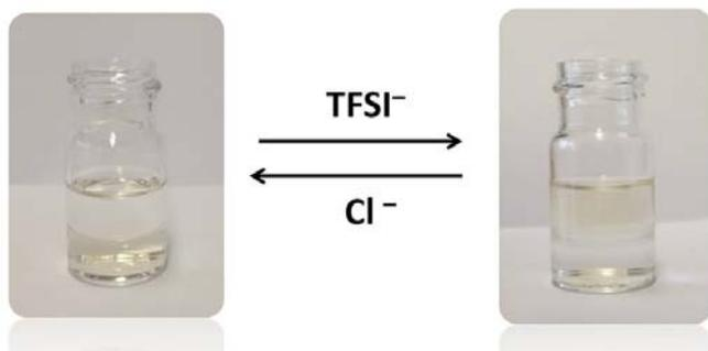
**Figure S25.** Photographs of the reversible phase transfer of Pt clusters assisted by the cage molecules between an aqueous and EA phases upon anion exchange.
