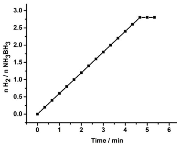
**Figure S32.** The time course plot of H<sub>2</sub> generation for Pt/RCC3 catalyst.
