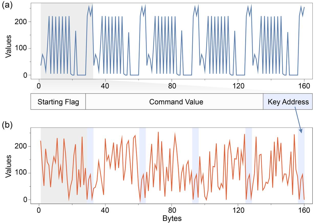
Supplementary Figure 1: **Intercepted commands before and after encryption.** (a) The plaintexts of five-time repeated commands. The inserted represents the structure of a command. (b) The ciphertexts of five-time repeated commands. Shadows mark the key information in each commands.
