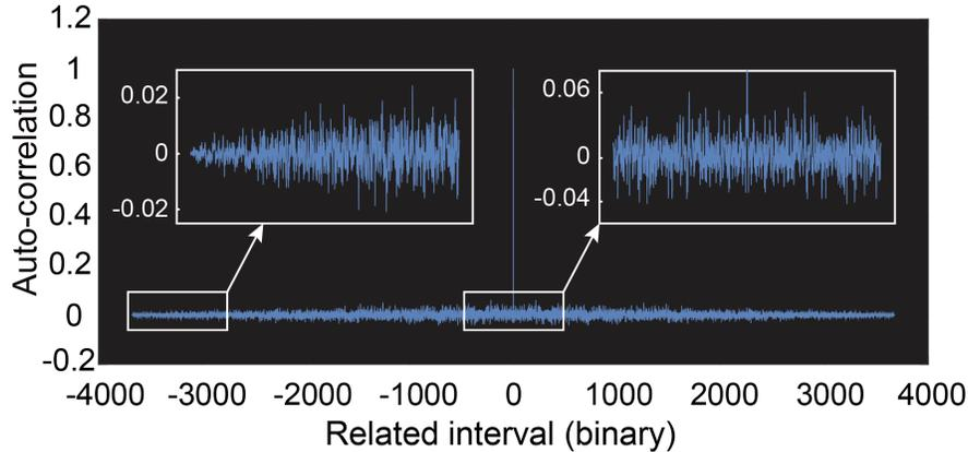
FIG. 3: **The auto-correlation function measured among long commands ciphertexts.** The auto-correlation function of ideal random sequence is close to delta function. The sharp auto-correlation peak in the center indicates that the encrypted binary sequence has excellent independence on each part. The insets show auto-correlation details in the near- and far-field regime.
