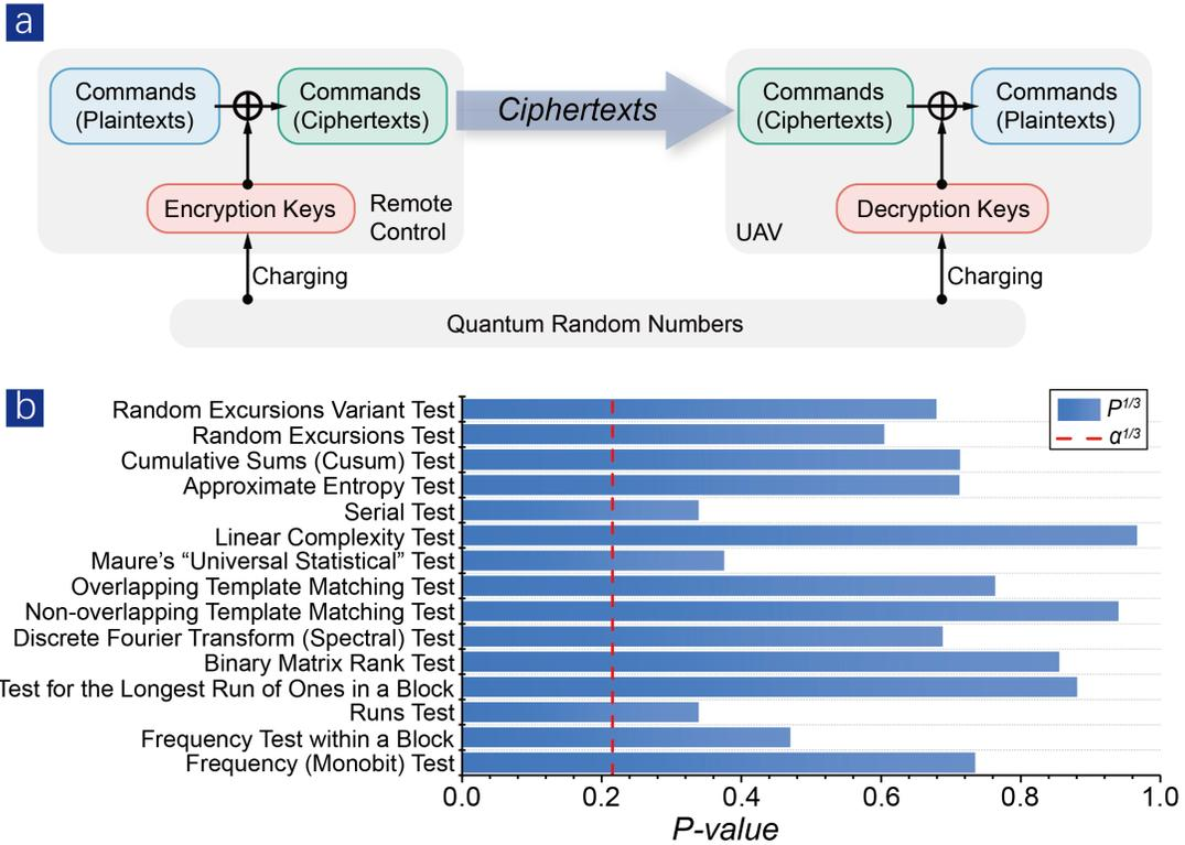
FIG. 2: **Signal flow diagram and NIST tests of quantum randomness.** (a) Signal flow diagram of the quantum-enhanced cryptographic control system. (b) NIST statistical randomness tests performance of quantum keys. The experimental results are obtained from 1,638,400 bits samples with a significance level of  $\alpha = 0.01$ . In the histogram, the value of each test that exceeded the red dashed line turns out a successful pass.
