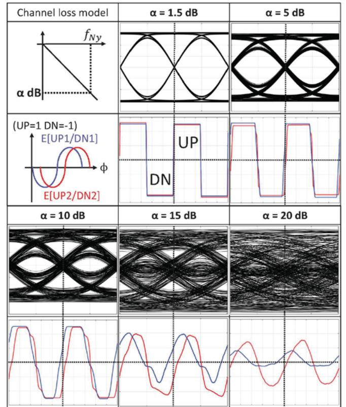
Fig. 4. Simulation results of two BBPD output groups classified by the exclusive-OR of two data bits
