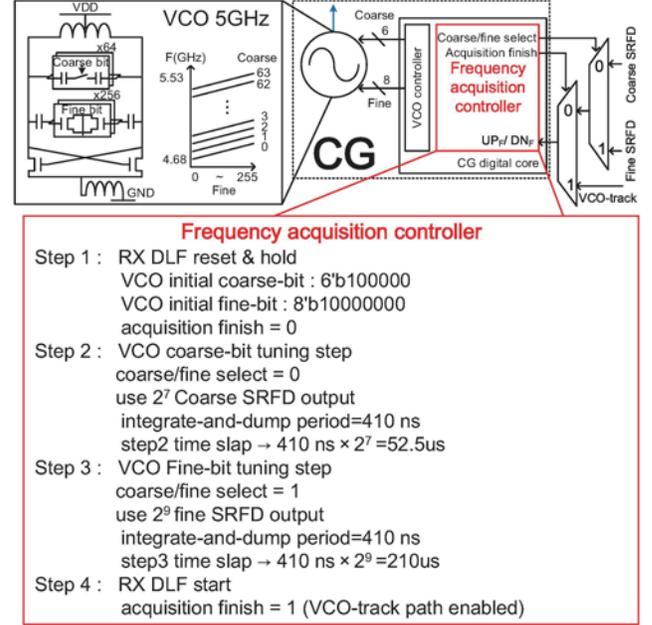
Fig. 7. The block diagram of Clock generator and frequency acquisition steps
