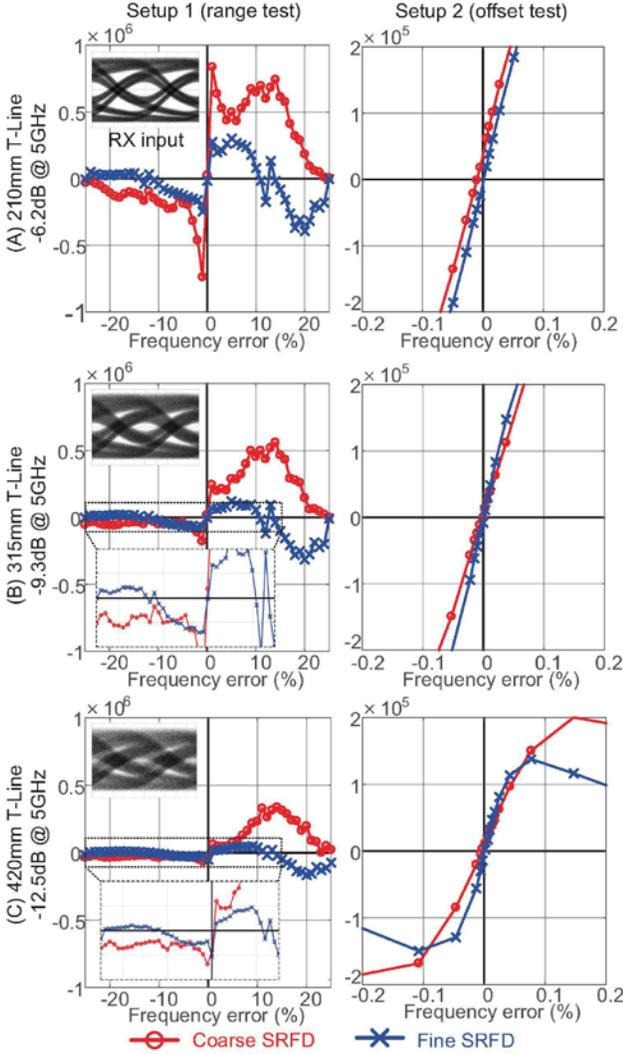
Fig. 8. Measured open loop output of type 2 dispersion-based SRFD
