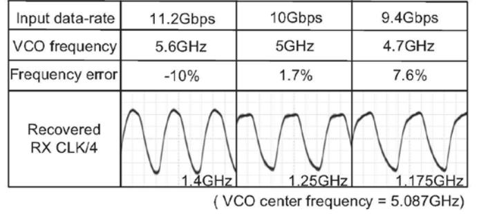
Fig. 9. RX clock recovered by the proposed frequency acquisition procedure
