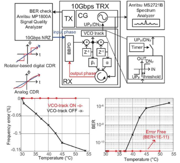
Fig. 10. Measured BER and VCO frequency versus chip temperature with and without VCO-track path
