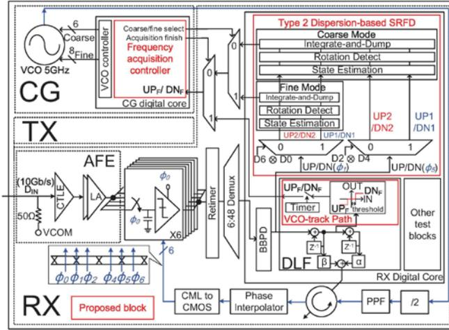
Fig. 6. The block diagram of 10Gbps reference-less transceiver
