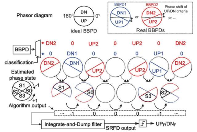
Fig. 1. Basic principle of SRFD algorithm
