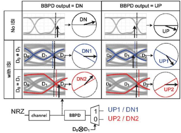
Fig. 3. The classification of BBPD output using inter-symbol interference (ISI)
