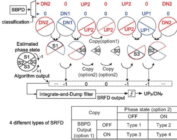
Fig. 2. 4 types of SRFD algorithm
