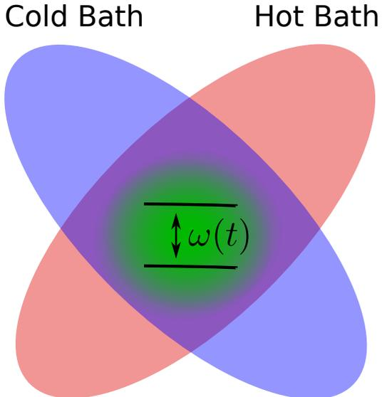
Figure 1: **A two-level system thermal machine:** Schematic setup showing a two-level system with periodically modulated level distance  $\omega(t)$  as the working fluid (WF) in a thermal machine wherein the WF is simultaneously coupled to hot and cold baths with non-overlapping spectra. Possible realizations include a driven-atom WF coupled to filtered heat baths in a cavity or a driven impurity coupled to spectrally distinct phonon baths in a solid structure [40, 41].
