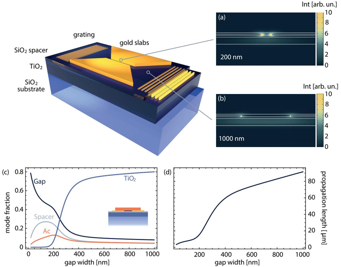
Figure 1. Schematic of the HGPW showing the layer structure. The two insets show the calculated intensity profiles of light in the HGPW for a gold gap of (a) 200 nm and (b) 1000 nm. (c) Distribution of the mode energy across the layers, as a function of channel gap width. The inset shows the various areas of the device considered. (d) Propagation length of the hybrid mode, again as a function of channel gap width.
