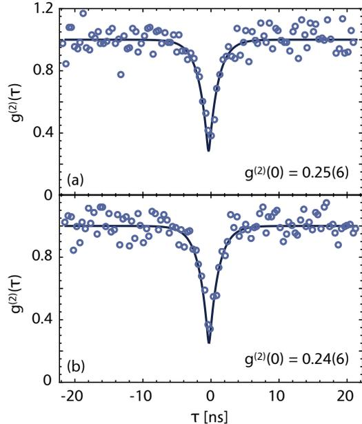
Figure 4. Correlation functions  $g^{(2)}(\tau)$  for the DBT fluorescence. (a) Auto-correlation of light collected directly from the molecule through the confocal microscope after a beamsplitter. (b) Cross-correlation of light collected from the left grating and from the confocal microscope. Dots show data. Solid curves are fits using Eq. 2. In both cases  $g^{(2)}(0)$  is well below 0.5 showing clear anti-bunching.
