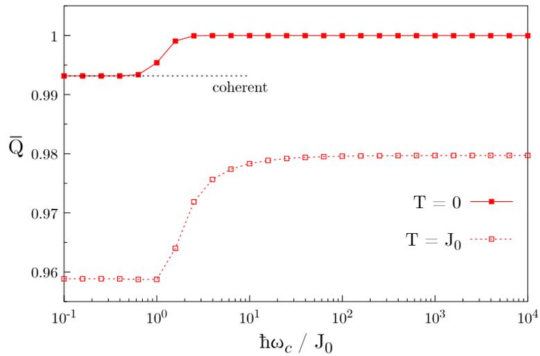
**Figure A2.**  $\bar{Q}$  vs the cutoff frequency  $\omega_c$  in the bath spectral function, at  $\tau = 20 \hbar/J_0$  and at bath temperatures  $T = 0, J_0$ . The horizontal dashed line indicates the value of  $Q_d^{\text{coh}}$ , the pumped charge at stationarity for the coherent dynamics, at the same  $\tau$ .
