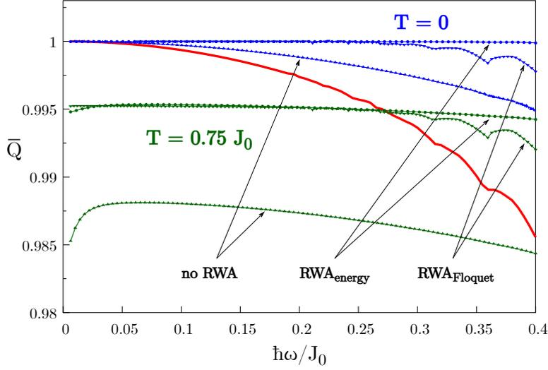
**Figure B1.**  $\bar{Q}$  vs driving frequency  $\omega$  for the dynamics induced by the Bloch-Redfield equation under different approximations. For all the cases, we still find a remarkable improvement over the coherent results if  $T$  is low enough. Notice, in particular, the good agreement between the two different RWA schemes.
