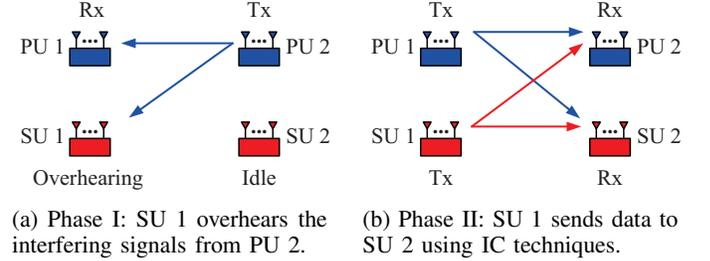
Fig. 4: Illustration of our proposed spectrum sharing scheme.
