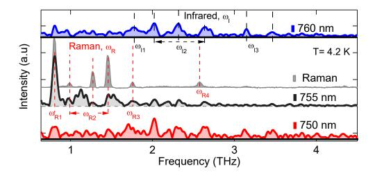
Figure 3. Fourier spectra of three  $\Delta R/R$  dynamics in Figs. 2(c)-(e), shown together with the static Raman spectrum (gray shade) at 4.2 K. Note the pronounced Raman mode  $\omega_{R1} \sim 0.8$  THz and IR phonon mode  $\omega_{I1} \sim 2$  THz. The assignment and symmetry analysis of other Raman and IR modes are shown in Fig. S6 (supplementary).
