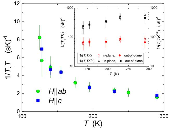
FIG. 5: Temperature dependence of  $^{139}\text{La}$   $1/T_1T$  for  $H\parallel ab$  (green circles) and  $H\parallel c$  (blue squares). The inset shows the semi-log plots of  $1/(T_1TK_s^2)$  and  $1/(T_1TK_s^{3/2})$  for two different magnetic fluctuation directions (in-plane and out-of-plane directions).
