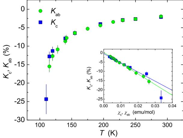
FIG. 4: Temperature dependence of  $^{139}\text{La}$  Knight shift for both  $H\parallel ab$  (green) and  $H\parallel c$  (blue) directions measured at  $H \sim 7$  T. Inset:  $K_{ab}$  vs.  $\chi_{ab}$  and  $K_c$  vs.  $\chi_c$  plots. The solid lines are linear fits as described in the text.
