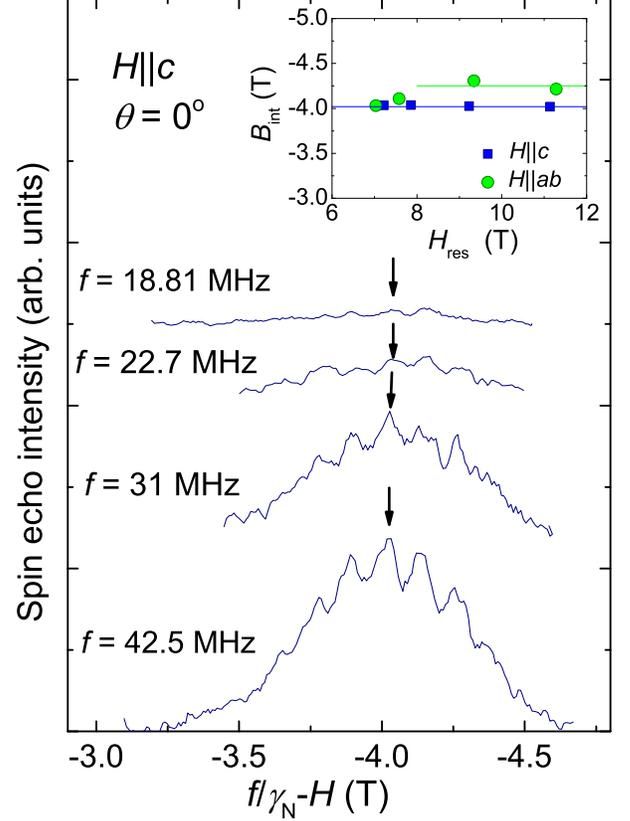
FIG. 3: (a)  $^{139}\text{La}$  NMR spectra at various frequencies for  $H||c$  at  $T = 1.65$  K. Inset: Resonance magnetic field ( $H_{\text{res}}$ ) dependence of  $B_{\text{int}}$  for  $H||ab$  (green circles) and  $H||c$  (blue squares). The arrows show the positions of the central transition line of the spectra measured at different frequencies
