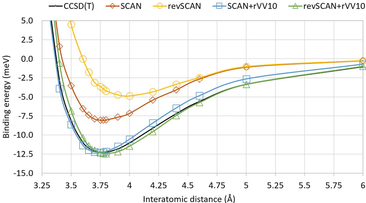
Figure 1: The binding energy curve of the Ar dimer from SCAN, revSCAN and their corresponding rVV10 corrected versions with respect to CCSD(T) curve. The value of  $b$  for SCAN+rVV10 and revSCAN+rVV10 are 15.7 and 9.4, respectively.
