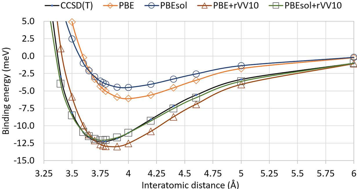
Figure 2: The binding energy curve of the Ar dimer from PBE, PBEsol and their corresponding rVV10 corrected versions with respect to CCSD(T) curve. The value of  $b$  for PBE+rVV10 and PBEsol+rVV10 are 9.8 and 9.7, respectively.
