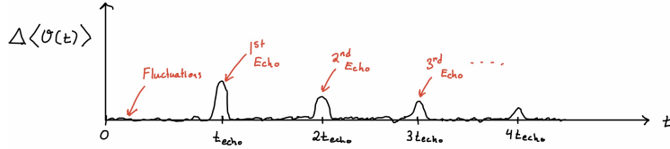
Figure 6. A diagram depicting how echoes will manifest themselves in a calculation involving \Delta \langle \hat{O}(t - t_0) \rangle . Initially, the difference in the expectation value of the operator is subject to small fluctuations around zero. After one echo time scale, one would find a distinct signal above the usual fluctuations represented by the first peak. This signals the first echo in the bulk. This would reflect off the boundary and go back towards horizon and the process would repeat except subsequent echoes would gradually weaken (depicted by subsequent peaks with smaller amplitude).
