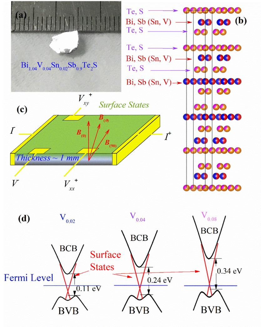
Fig. 1 Atomic and electronic structures of single crystal V:BSSTS. (a) Typical size of  $V_{0.04}$  doped single crystal exfoliated from the as-grown ingot. (b) A sketch of the van der Waals layers in the V:BSSTS single crystal. (c) Schematic diagram of the transport measurement geometry for measuring a freshly-cleaved V:BSSTS surface. Note that, during tilting, the magnetic field is always perpendicular to the electronic current. (d) Possible bulk band structures in V:BSSTS single crystals.
