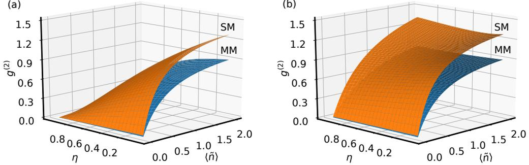
**Figure 2.** The  $g^{(2)}$ -function of the heralded target state calculated via Eq. (5), when conditioned with a measurement of (a) one photon with a photon-number-resolving detector and (b) a single click with a bucket detector in the herald. Since the latter can only resolve between *click* and *no click*, it heralds in all cases in which one or more photons impinge on it. Orange and blue surfaces as labeled in the figure illustrate the behavior of SM and MM PDC emission, respectively.
