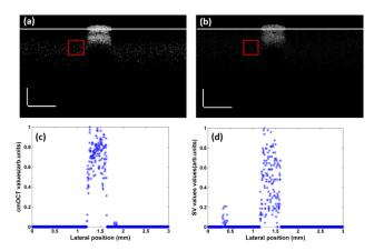
Fig. 3. (a) cmOCT image obtained from the transverse scan shown in Fig. 2(a) with static region of interest marked in red, (b) corresponding SV image with static region of interest marked in red (c) Profile plot obtained over the marked line in (a), (d) Profile plot obtained over the marked line in (b) (scale bar is  $500 \,\mu$ m).
