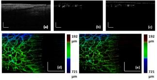
Fig. 4. (a) Representative B-scan image of the little finger of adult volunteer, (b) corresponding cmOCT image, (c) corresponding SV image (d) depth encoded intensity projection image of enface cmOCT images, (e) depth encoded intensity projection image of enface SV images (scale bars in x and y directions are 500  $\mu$ m).
