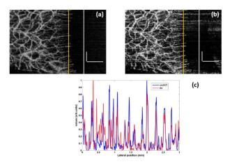
Fig. 5. (a) MIP of enface cmOCT images from nailfold (b) MIP of SV enface images (c) signal profiles extracted from the position marked in yellow in (a) and (b); Scalebars are  $500 \mu m$ .
