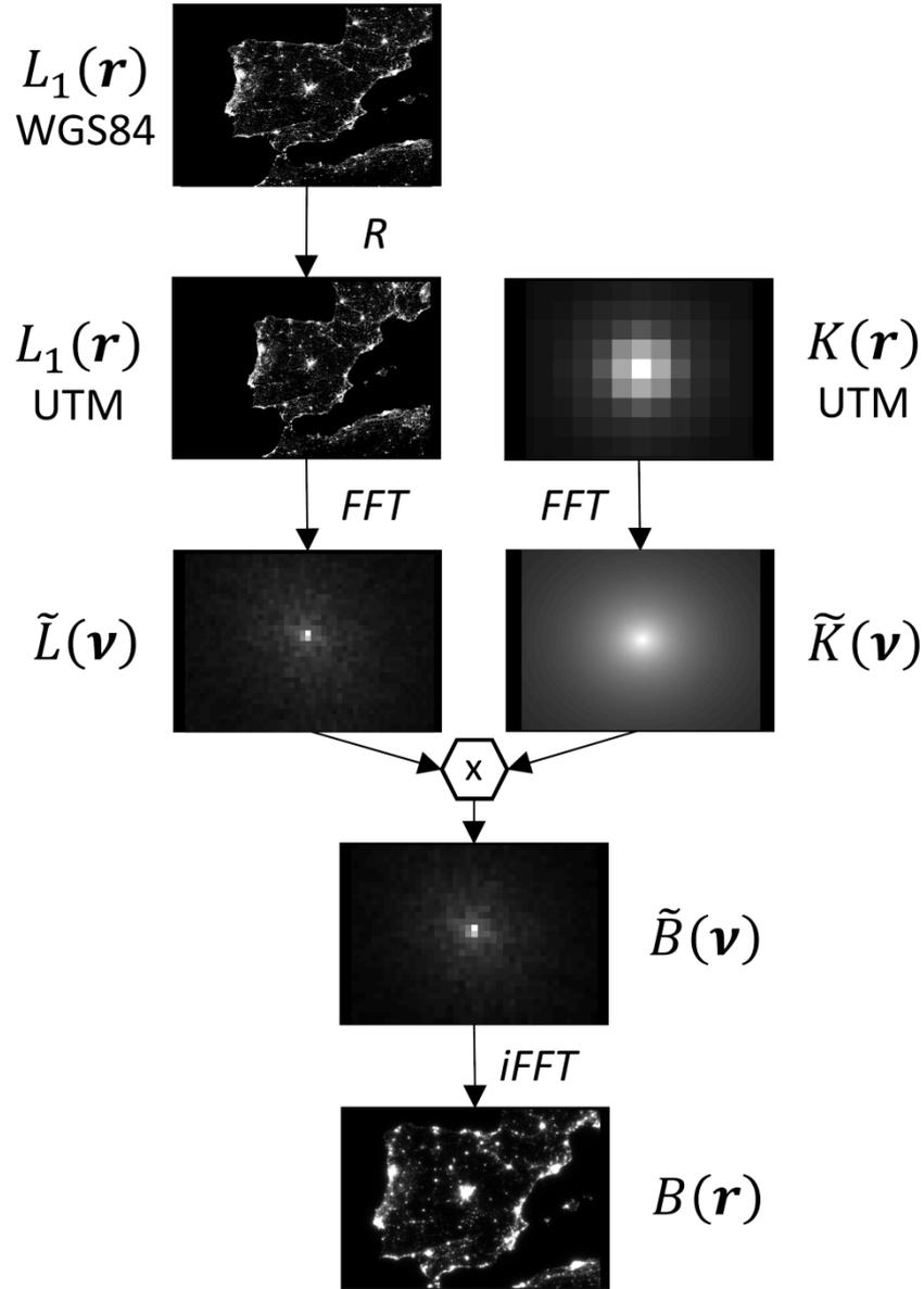
**Figure 1:** Steps for calculating light pollution maps using the Fourier convolution theorem.  $R$ : map reprojection;  $FFT$ : Fourier-transform;  $iFFT$ : inverse Fourier-transform.  $\tilde{B}(\mathbf{v})$ ,  $\tilde{K}(\mathbf{v})$ , and  $\tilde{L}(\mathbf{v})$  are in general complex functions; their absolute values are plotted in this figure.
