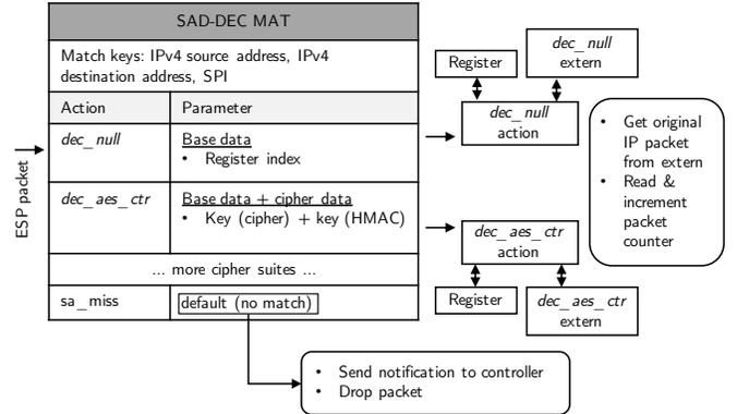
Fig. 12. ESP decryption function block. ESP packets are processed by a SAD-DEC MAT. It holds entries for each SA with the corresponding data that is required for applying the associated cipher suite externs for decryption.
