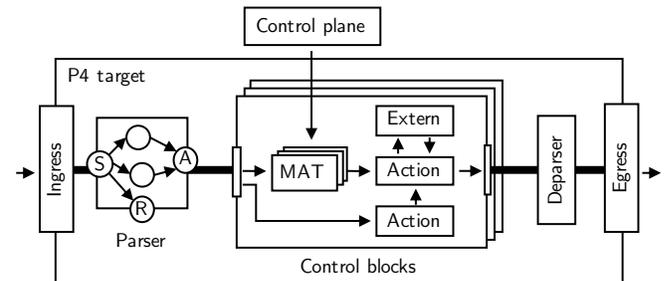
Fig. 5. Simplified view on the P4 processing pipeline of P4<sub>16</sub>. It comprises the parser, control blocks, and the deparser. Each control block may include MATs, actions, and externs.
