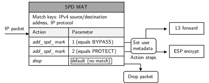
Fig. 10. SPD matching function block. IP packets are processed by the SPD MAT. The *add\_spd\_mark* action adds the given parameter to the user metadata of the packet. It decides if the packet is protected by IPsec (PROTECT) or forwarded without protection (BYPASS) in later stages.
