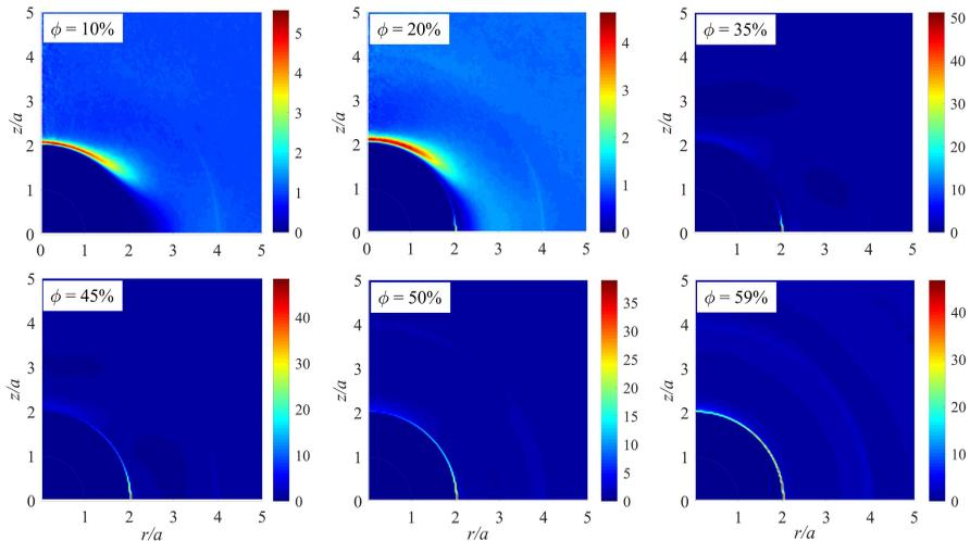
FIGURE 3. Pair distribution functions in the suspensions undergoing dipolophoresis at six different volume fractions in cylindrical coordinates  $(r, z)$ , where  $r^2 = x^2 + y^2$ . A probe particle is located at the origin.
