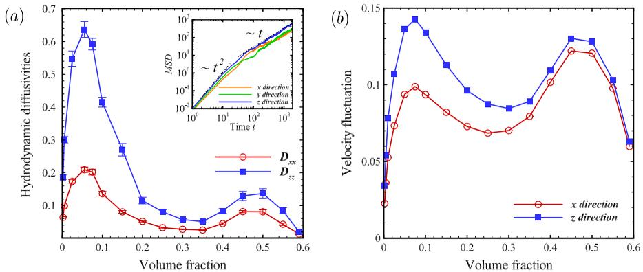
FIGURE 2. (a) Hydrodynamic diffusivities in the transverse direction ( $x$ ) and the field direction ( $z$ ) versus volume fractions with the error bars based on the block-averaging method (Flyvbjerg & Petersen 1989). Inset: mean-square displacement (MSD) curves in the transverse ( $x$ ,  $y$ ) and field direction ( $z$ ) at  $\phi = 50\%$  as functions of time on a log-log scale. (b) Standard deviations of particle velocities as functions of volume fraction in the  $x$  and  $z$  directions.
