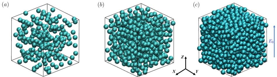
FIGURE 1. Snapshots of particle distributions in a periodic cell of dimensions  $L_x \times L_y \times L_z = 20^3$  at different volume fractions: (a)  $\phi = 10\%$  (dilute), (b)  $\phi = 25\%$  (semi-dilute), and (c)  $\phi = 59\%$  (concentrated). Also see the accompanying online movies.
