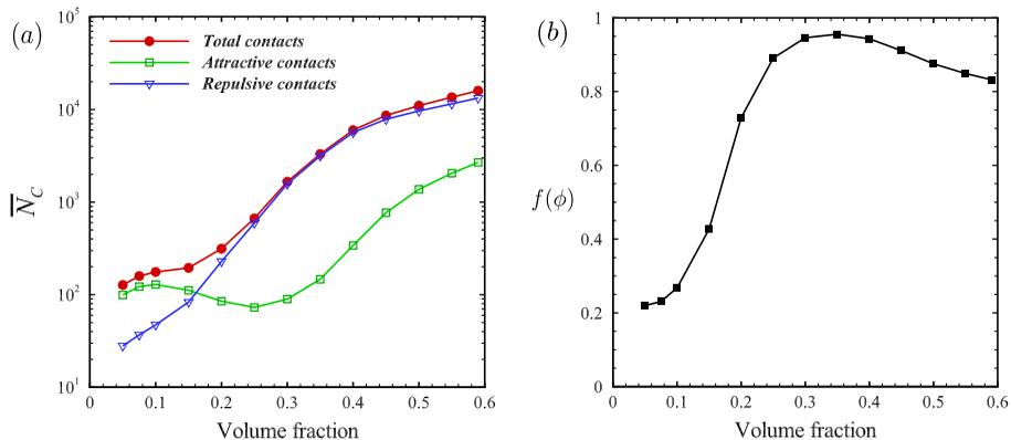
FIGURE 6. (a) The time-averaged number of total contacts, attractive contacts, and repulsive contacts as functions of volume fraction. (b) The contact ratio  $f$ , which is the fraction of the number of repulsive contacts to total contacts, as a function of volume fraction.
