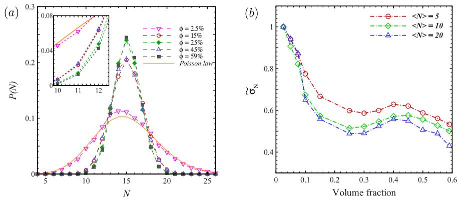
FIGURE 4. (a) Particle occupancy distributions for  $\langle N \rangle = 15$  at different volume fractions along with a Poisson distribution. (b) The standard deviations of number-density fluctuations normalized with their maximum value as functions of volume fraction for three expected values  $\langle N \rangle = 5, 10, 20$ .
