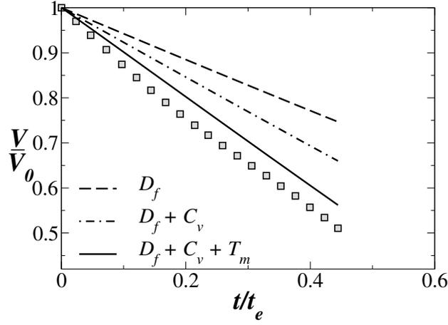
FIG. 22: Comparison of the experimental and theoretically obtained  $(V/V_0)$  versus  $t/t_e$  at  $T_s = 60^\circ\text{C}$  for pure ethanol (E 100% + W 0%) calculated using diffusion ( $D_f$ ), diffusion + convection ( $D_f + C_v$ ) and diffusion + convection + transport ( $D_f + C_v + T_m$ ) models.
