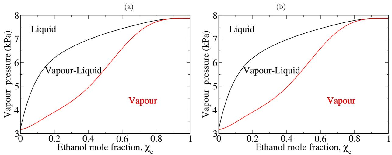
FIG. 19: The vapour-liquid pressure curves for the binary mixture at (a) 25°C and (b) 60°C [50].
