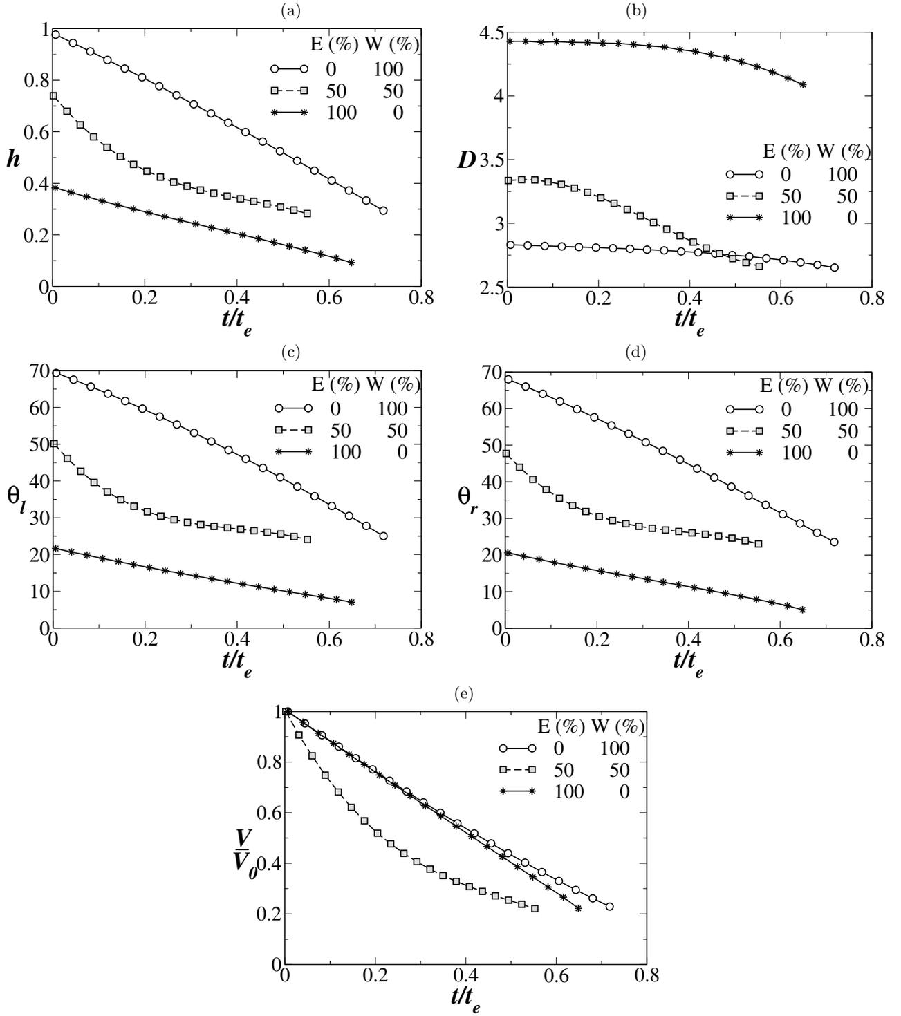
FIG. 8: Variations of (a) the height ( $h$ ) in mm, (b) the wetting diameter of the droplet ( $D$ ) in mm, (c) the left contact angle ( $\theta_l$ ) in degree, (d) the right contact angle ( $\theta_r$ ) in degree and (e) the normalised volume with the initial volume of the droplet ( $V/V_0$ ) versus time normalised with the lifetime of the droplet ( $t/t_e$ ) for different ethanol (E) - water (W) compositions at  $T_s = 25^\circ\text{C}$ .
