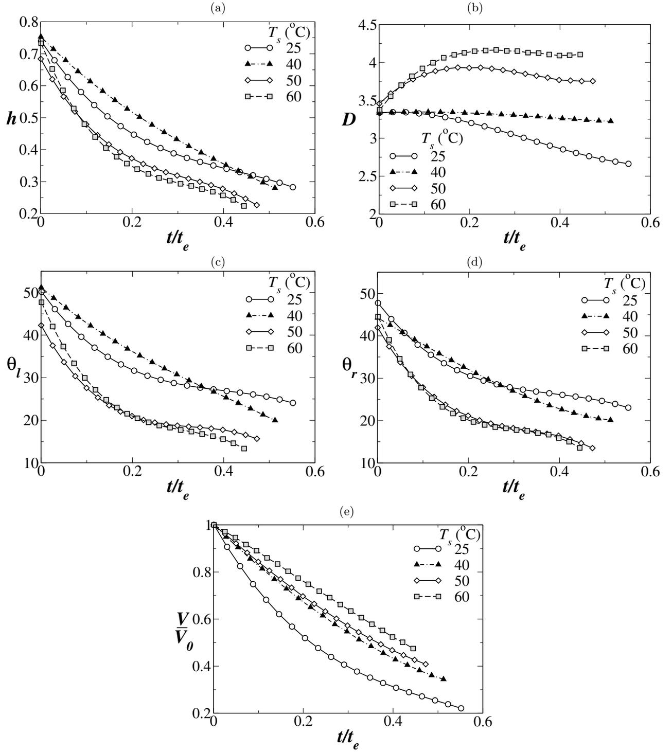
FIG. 17: Variations of (a) the height ( $h$ ) in mm, (b) the wetting diameter of the droplet ( $D$ ) in mm, (c) the left contact angle ( $\theta_l$ ) in degree, (d) the right contact angle ( $\theta_r$ ) in degree and (e) the normalised volume with initial volume of the droplet ( $V/V_0$ ) versus time normalised with the life time of the droplet ( $t/t_e$ ) at different substrate temperatures for (E 50% + W 50%) solution.
