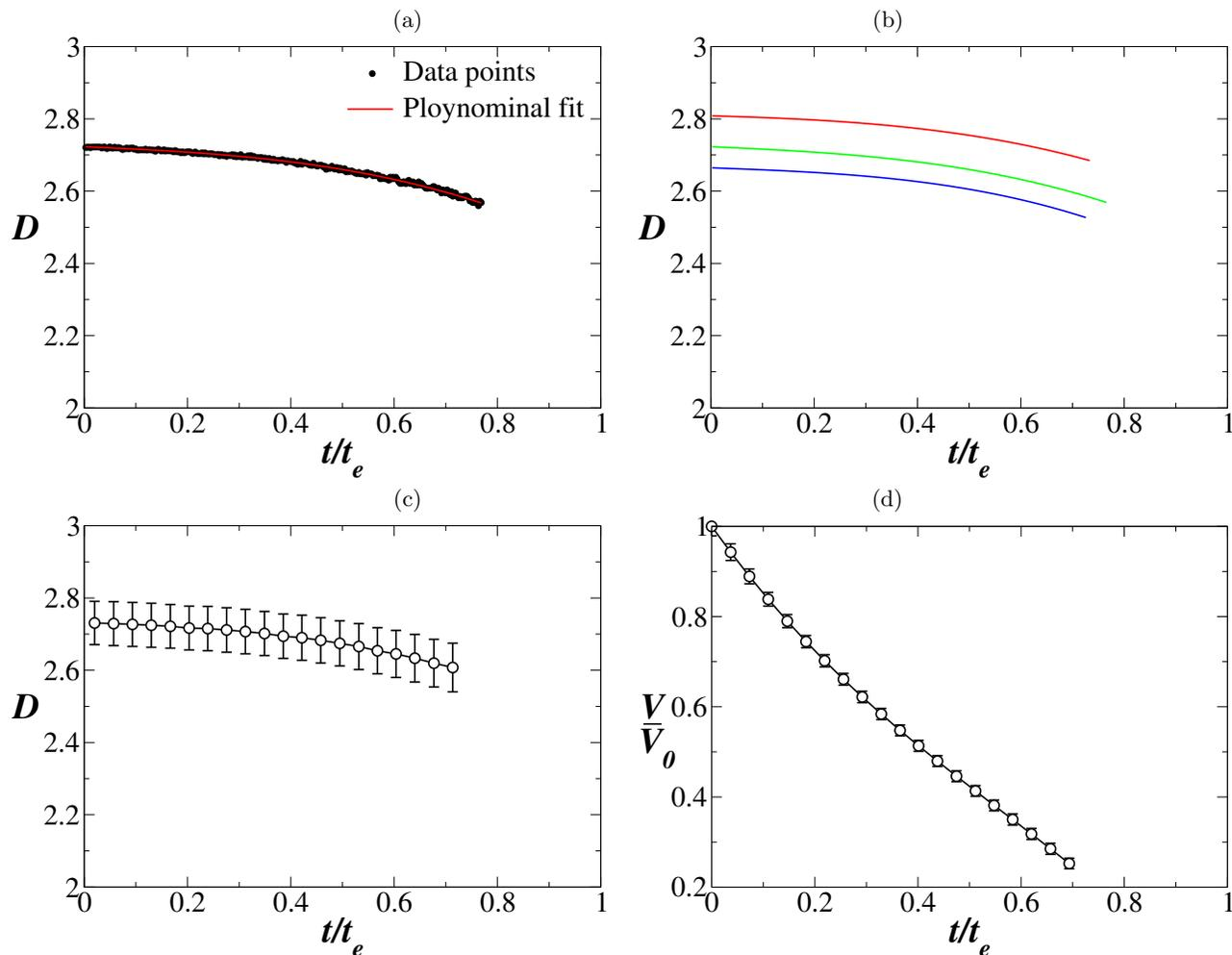
FIG. 5: The steps associated with the data processing for a typical droplet. (a) The typical data points for the diameter of the droplet,  $D$  (mm) versus  $t/t_e$  for one recording video and the polynomial fit, (b) the polynomial fits for three repetitions, (c) the resultant polynomial fit with an error bar and (d) the final  $V/V_0$  versus  $t/t_e$  plot.
