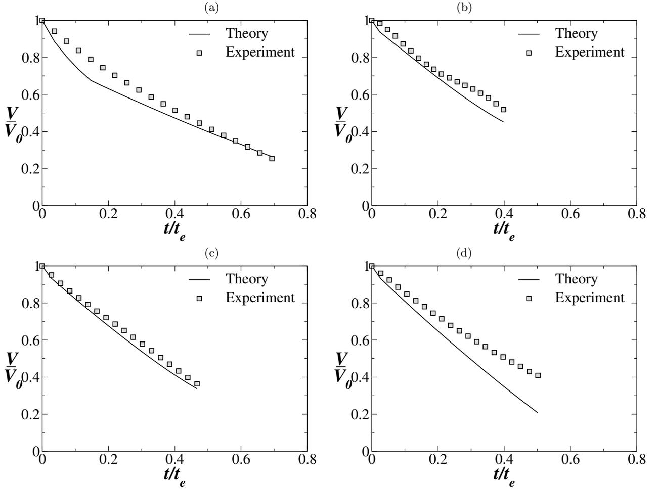
FIG. 23: Comparison of the experimental and theoretically obtained  $(V/V_0)$  versus  $t/t_e$  at  $T_s = 60^\circ\text{C}$  for droplet of binary mixtures (a) (E 20% + W 80%), (b) (E 50% + W 50%), (c) (E 60% + W 40%) and (d) (E 80% + W 20%).
