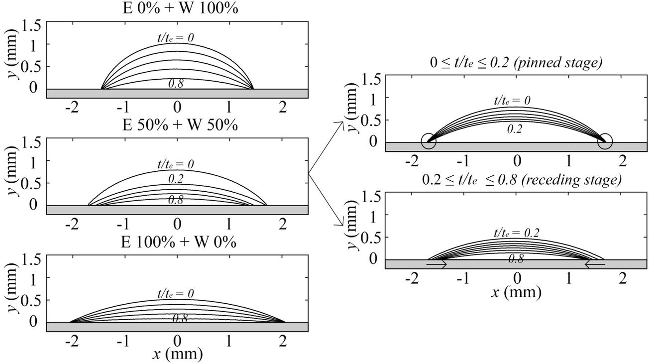
FIG. 7: Contours of the droplet for pure water (E 0% + W 100%), (E 50% + W 50%) solution and pure ethanol (E 100% + W 0%) at different normalised times,  $t/t_e$ . The contours are plotted at an interval of 0.2. The substrate temperature,  $T_s$  is 25°C.
