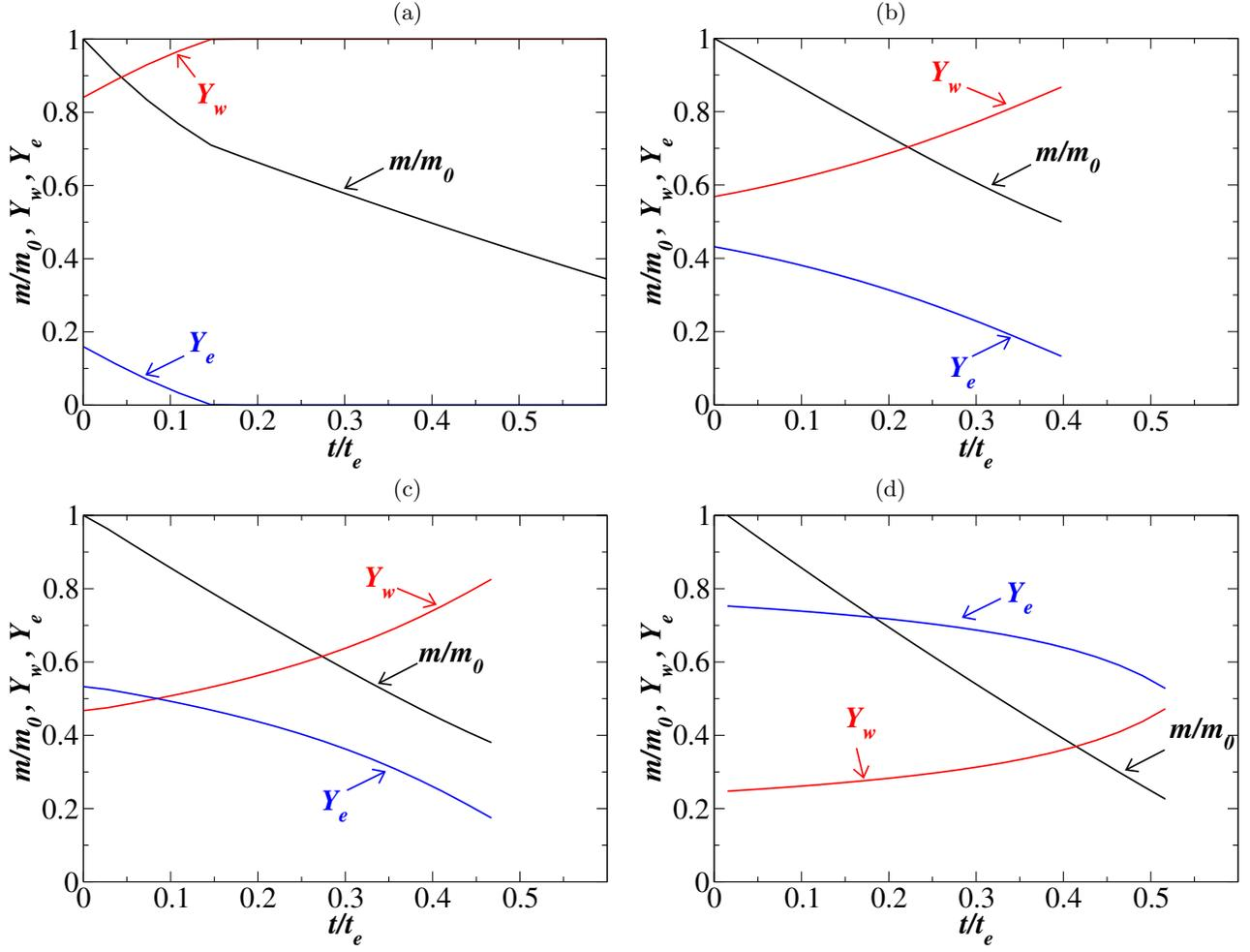
FIG. 24: The variations of normalised mass of the droplet with the initial mass of the droplet ( $m/m_0$ ),  $Y_w$  and  $Y_e$  versus  $t/t_e$  at  $T_s = 60^\circ\text{C}$  for droplets of (a) (E 20% + W 80%), (b) (E 50% + W 50%), (c) (E 60% + W 40%) and (d) (E 80% + W 20%).
