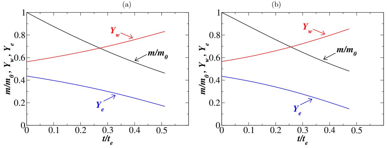
FIG. 26: The variations of the normalised mass of the droplet with the initial mass of the droplet ( $m/m_0$ ), water and ethanol mass fractions,  $Y_w$  and  $Y_e$  versus  $t/t_e$  at different substrate temperatures for a droplet of (E 50% + W 50%) binary mixture. (a)  $T_s = 40^\circ\text{C}$  and (b)  $T_s = 50^\circ\text{C}$
