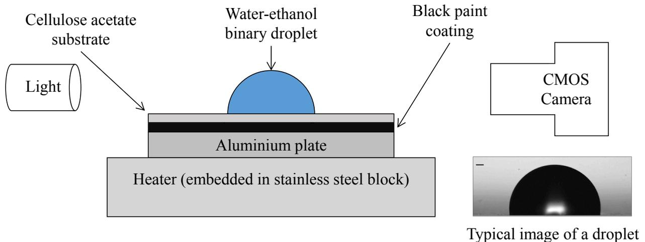
FIG. 1: Schematic diagram of the experimental set-up. It consists of a heater, a cellulose acetate substrate placed on a stainless steel plate, a light source and a camera. A typical image of an ethanol-water droplet recorded using a CMOS camera is also shown.
