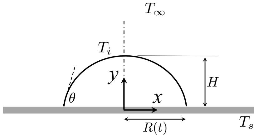
FIG. 18: Schematic diagram of a sessile droplet on a substrate maintained at temperature,  $T_s$ .  $H$  and  $R(t)$  are the height and the wetting radius of the droplet;  $\theta$  is the contact angle;  $T_i$  and  $T_\infty$  are the temperature at the liquid-vapour interface and the temperature of the ambient far away from the droplet, respectively.
