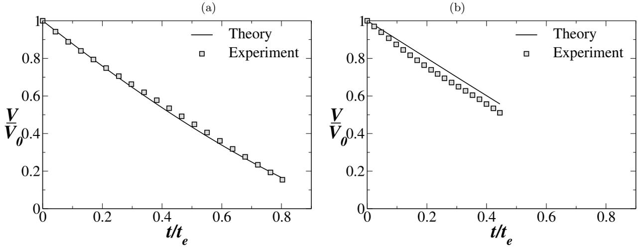
FIG. 21: Comparison of the experimental and theoretically obtained  $(V/V_0)$  versus  $t/t_e$  at  $T_s = 60^\circ\text{C}$  for pure fluids. (a) Pure water (E 0% + W 100%), and (b) pure ethanol (E 100% + W 0%).
