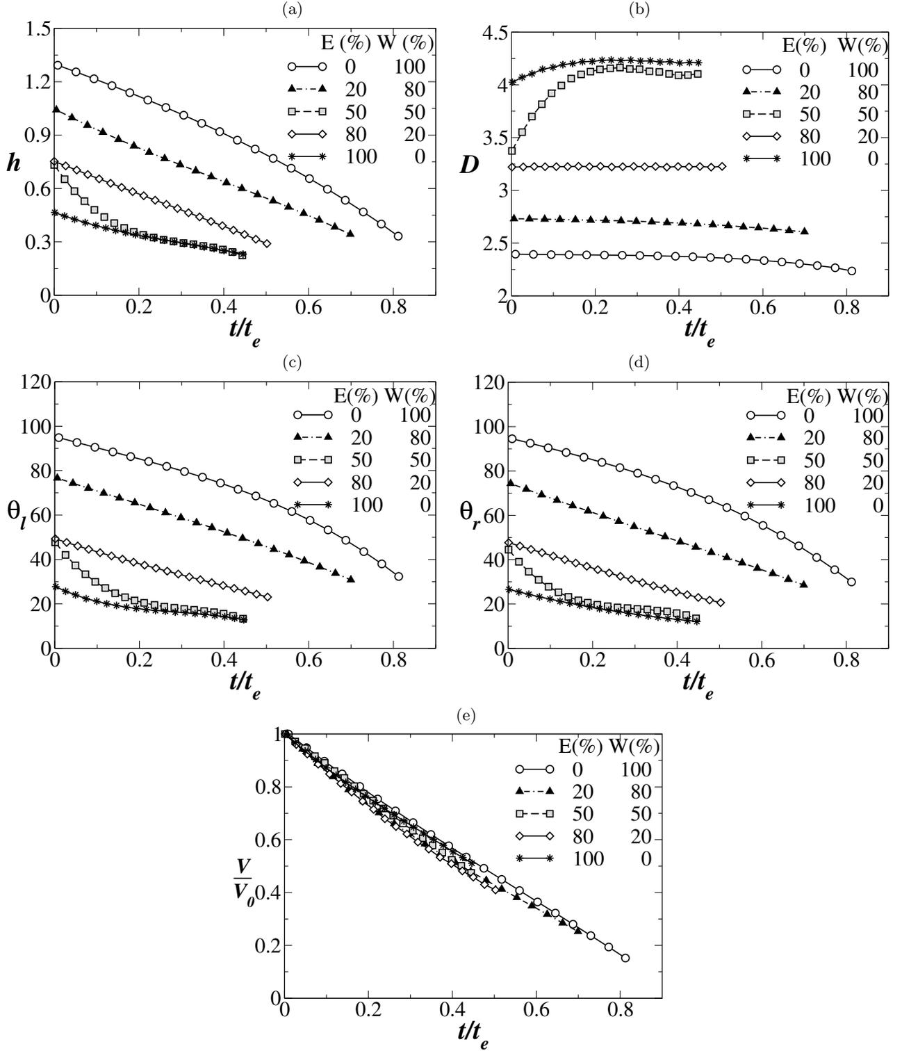
FIG. 13: Variations of (a) the height ( $h$ ) in mm, (b) the wetting diameter of the droplet ( $D$ ) in mm, (c) the left contact angle ( $\theta_l$ ) in degree, (d) the right contact angle ( $\theta_r$ ) in degree and (e) the normalised volume with initial volume of the droplet ( $V/V_0$ ) versus time normalized with the lifetime of the droplet ( $t/t_e$ ) for different ethanol (E) - water (W) concentration at  $T_s = 60^\circ\text{C}$ .
