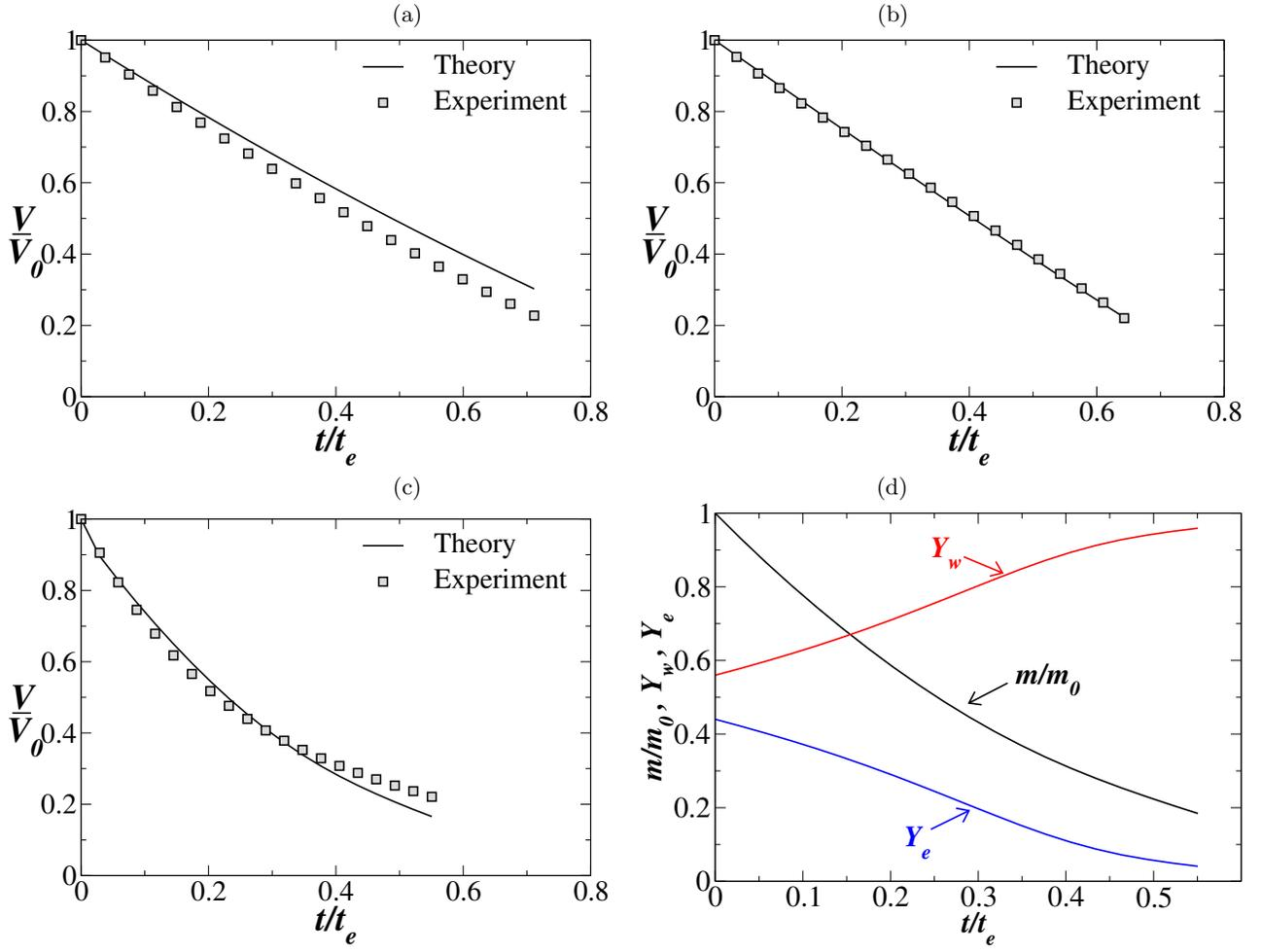
FIG. 20: Comparison of the experimental and the theoretically obtained  $(V/V_0)$  versus  $t/t_e$ . (a) Pure water (E 0% + W 100%), (b) pure ethanol (E 100% + W 0%) and (c) droplet of (E 50% + W 50%) binary mixture. (d) The variations of the normalised mass of the droplet with the initial mass of the droplet ( $m/m_0$ ), water and ethanol mass fractions,  $Y_w$  and  $Y_e$  versus  $t/t_e$ . Here substrate temperature,  $T_s$  is 25°C
