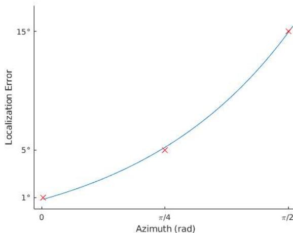
Figure 19: Simple fitted model of sound localization error by azimuth. The amount of noise imposed on  $\tilde{\theta}_m$  is set to be proportional to the localization error.
