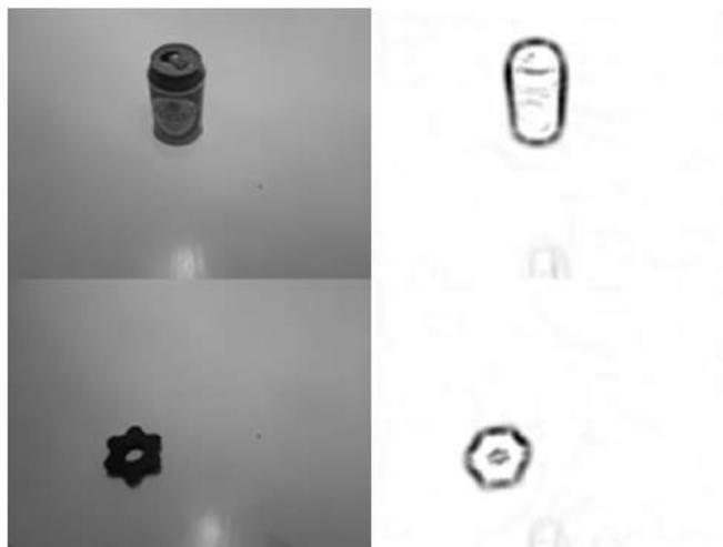
Figure 22: Example images and corresponding contour representations from the table dataset. A beer or a gear was placed in various positions on the table, while being recorded by a mounted mobile phone.
