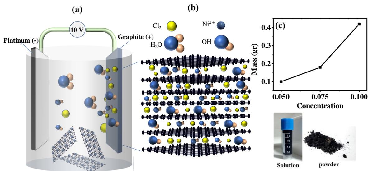
**Figure 1.** (a) Schematic illustration of the proposed mechanism for magnetic Gr/Ni production, (b) Situation of OH<sup>-</sup> and Cl<sup>-</sup> ions between graphite sheets which increases the interlayer distance. Cl<sup>-</sup> gas can exert excessive force to graphite layers which results in separation of the graphite layers and then Gr sheets distributed in the solution can trap Ni<sup>2+</sup> ions. (c) Concentration of electrolyte solution and final mass of magnetic Gr/Ni composite.
