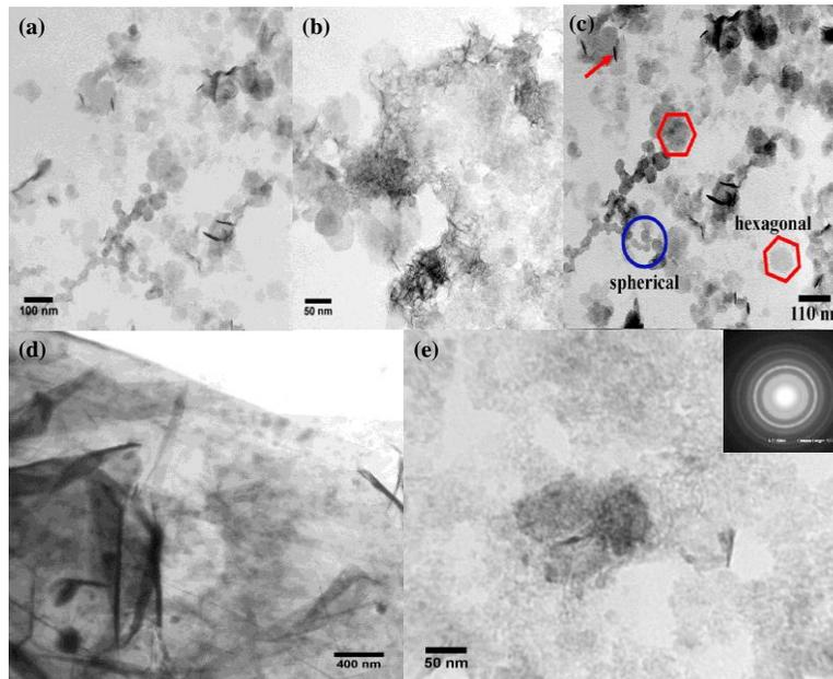
**Figure 4.** TEM images of (a) 0.1 M, (b) 0.075 M, (c) 0.05 M samples and (d) micron boundary size of Gr sheets and (e) SAED pattern of the 0.05 M sample.
