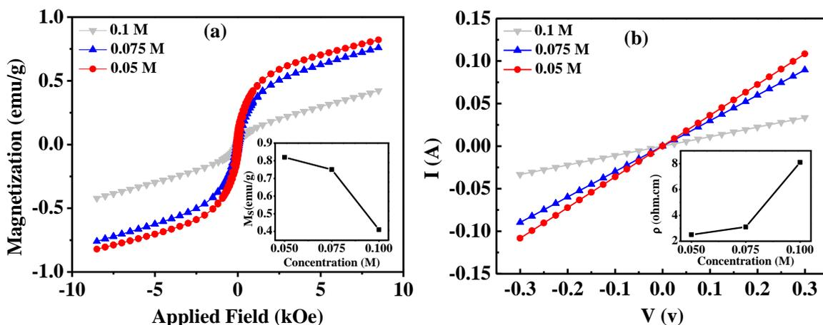
**Figure 5.** (a) VSM magnetization plots of 0.05 M, 0.075 M and 0.1 M samples. Inset shows the saturation magnetization of samples versus concentration. (b) Current-Voltage (I-V) curve measurement for 0.05 M, 0.075 M and 0.1 M samples and inset shows the resistivity ( $\rho$ ) of samples versus concentration.
