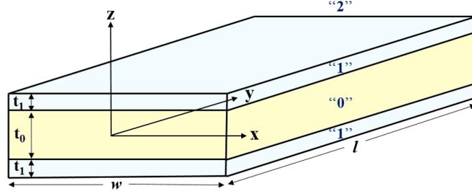
**Figure 7.** Schematic of the ribbon/GrNi structures and the coordinate system.
