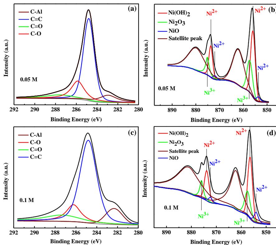
**Figure 3.** High-resolution XPS spectra of C 1s and Ni 2p core level of Gr/Ni sample of (a, b) 0.05 M and (c, d) 0.1 M.
