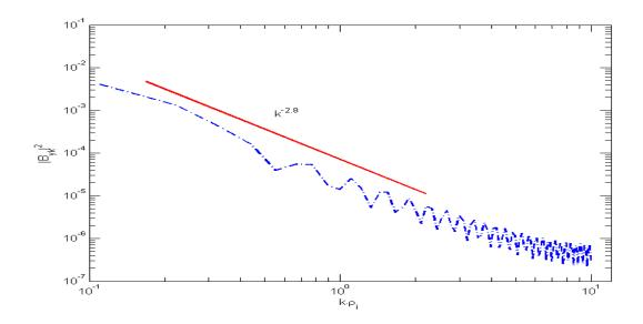
Figure 7. The magnetic field spectra obtained by the simulation. The variation of  $|B_{yk}|^2$  against k is depicted on the y-axis. The thick red line represents the spectral slope value.
