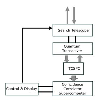
Figure 1. Block diagram of quantum radar design.
