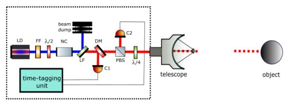
Figure 5. Schematic of the experimental setup to test the proof-of-principle quantum radar concept.
