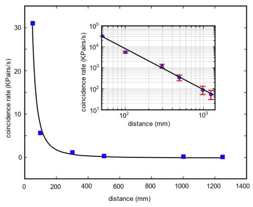
Figure 6. Cross-correlogram delay values are converted to distance. The solid black line shows the theoretical fit to the experimental data. The inset shows the logarithmic scale for the ease of reading.
