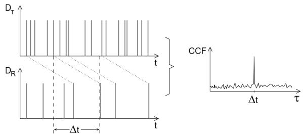
Figure 2. Extracting the target range by cross correlation of timing signals.
