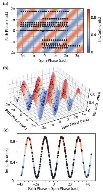
Fig 2 (a) The black circles indicate the path and spin phases where measurements were taken at a neutron wavelength of 0.4 nm. The colored stripes illustrate the cosine curve fitted to the data (b) 3D view of the normalized intensities (black circles) plotted against the path and spin phases and fitted by a cosine fitting function. (c) Measured intensities and the fitted cosine function plotted against the sum of path and spin phase. Error bars are the size of the markers or smaller.
