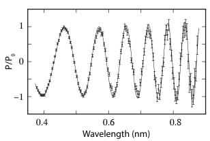
Supp Fig 1: Fit of the normalized neutron polarization as a function of neutron wavelength ( $\lambda_n$ ) as described in the Methods section. In this case, the energy phase deduced from the RF frequency was  $\gamma = -1.00\pi$ . The fitted value for the path phase is  $\chi = -1.06 \pi$  and for the spin plus energy phase is  $\alpha + \gamma = -2.01 \pi$ .
