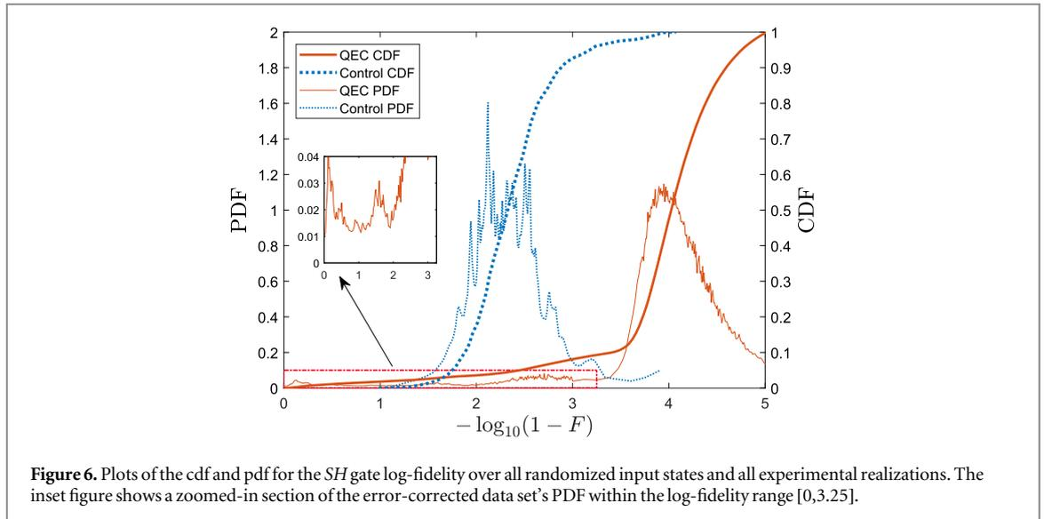
**Figure 6.** Plots of the cdf and pdf for the *SH* gate log-fidelity over all randomized input states and all experimental realizations. The inset figure shows a zoomed-in section of the error-corrected data set's PDF within the log-fidelity range [0,3.25].
