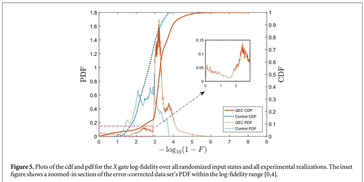
**Figure 5.** Plots of the cdf and pdf for the X gate log-fidelity over all randomized input states and all experimental realizations. The inset figure shows a zoomed-in section of the error-corrected data set's PDF within the log-fidelity range [0,4].
