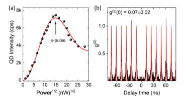
FIG. 4. (a) Resonance fluorescence intensity plotted versus the square root of the excitation power, recorded for QD-cavity detuning of  $\Delta$  = 180 µeV. The red solid line is a fit using a damped Rabi rotation model. (b) Second-order autocorrelation histogram as a function of delay time between subsequently emitted photons recorded under pulsed s-shell resonant excitation with a  $\pi$ -pulse area (223 nW). The red solid line is a two-sided exponential decay fit.
